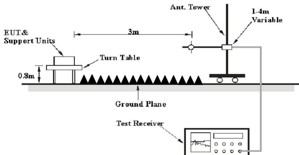
The radiated emission tests were performed in the 3 meters chamber test site, using the setup accordance with the FCC MP - 5. The specification used was the FCC part 18 limits.
