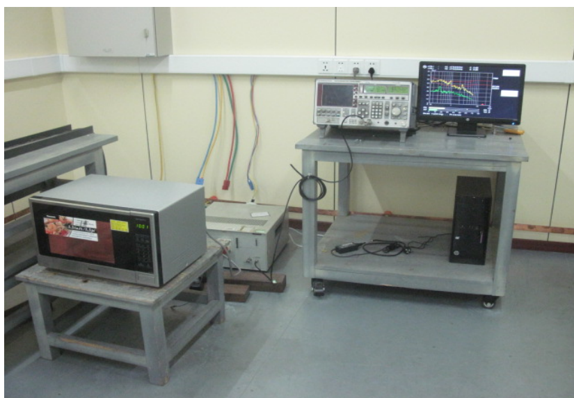
Conducted Emission Test Set-up
