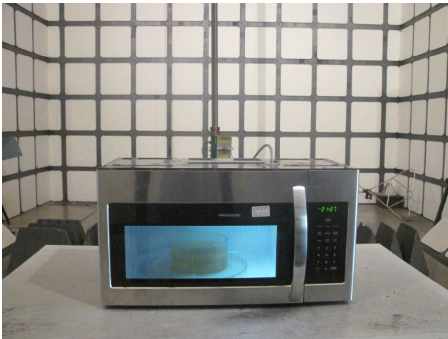
Operating Frequency Test Set-up
