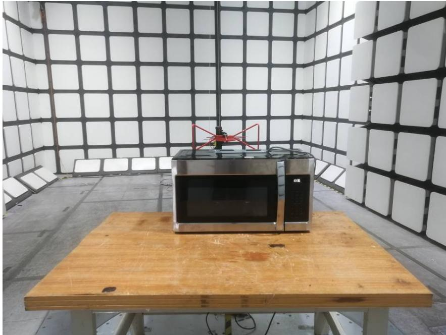
**Radiated Emissions - Rear View (30 MHz – 1 GHz)**
