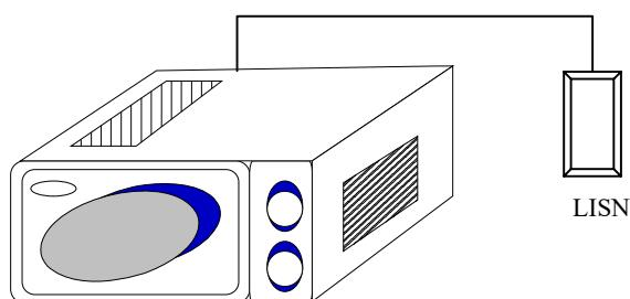
**Block Diagram of Test Setup**
