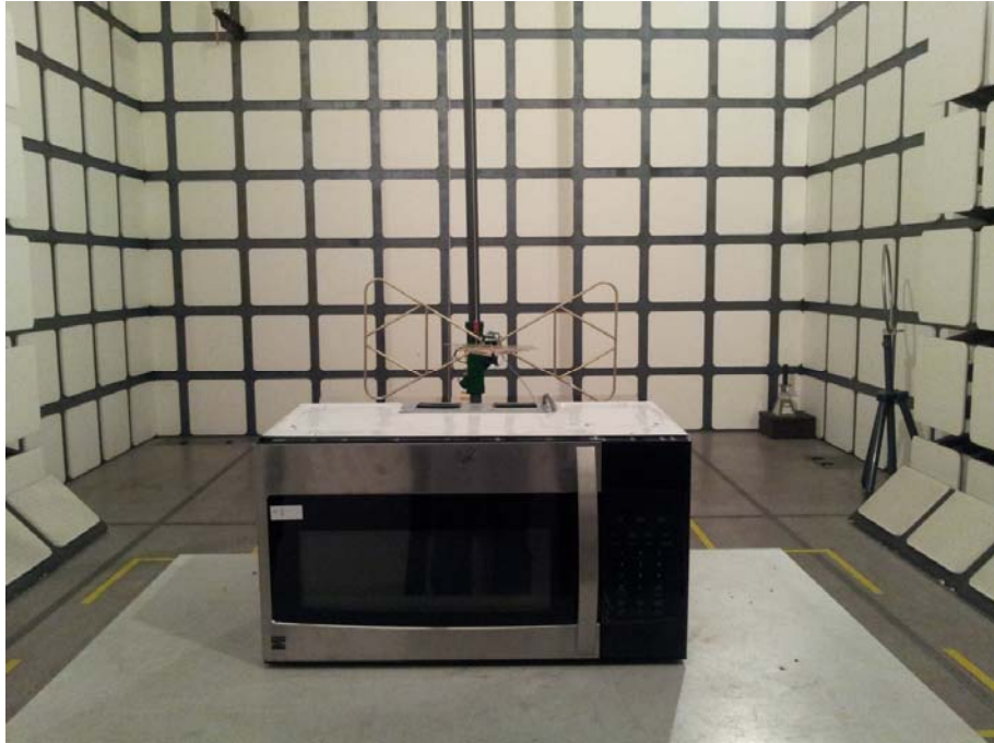
Radiated Emission Test Set-up (30 -1,000MHz)
