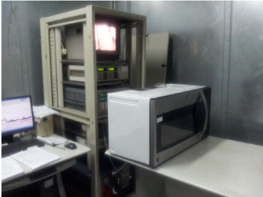
Conducted Emission Test Set-up
