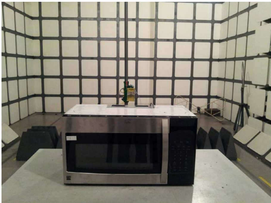
Radiated Emission Test Set-up (1-18GHz)
