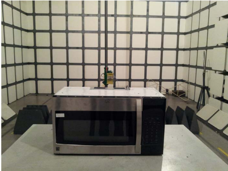
Operating Frequency Test Set-up
