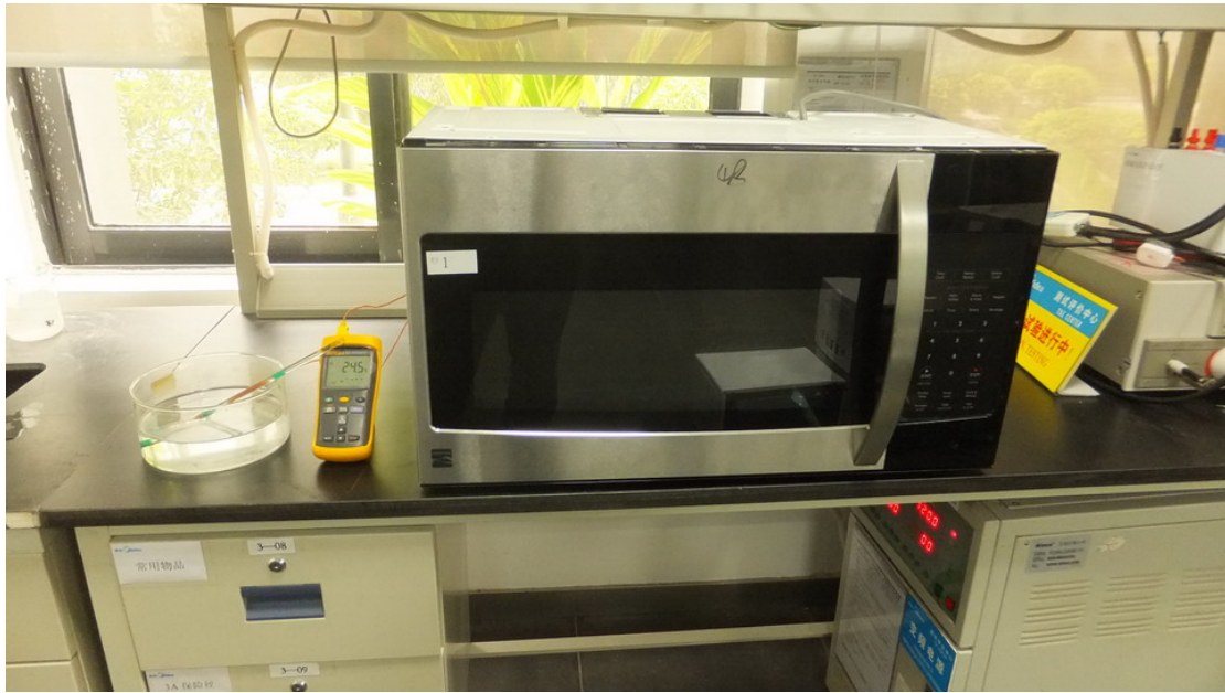
RF Output Power Test Set-Up
