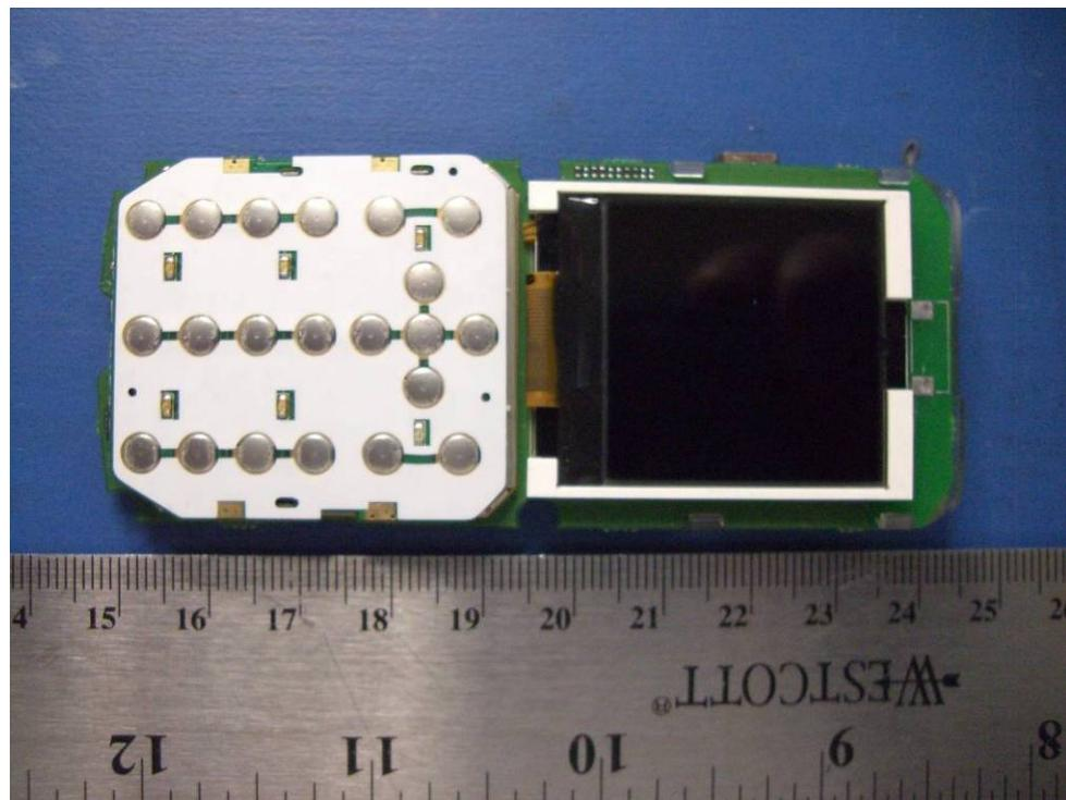
**EUT Internal PCB Component Side, Keyboard Removed**
