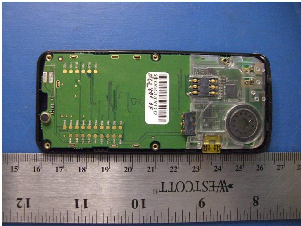
**EUT Internal PCB Component Side View with Keyboard & Display**
