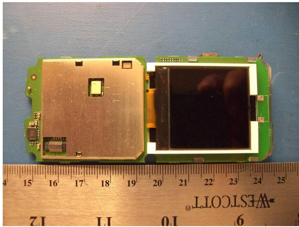
**EUT Internal PCB Component Side, RF Shielding Removed**
