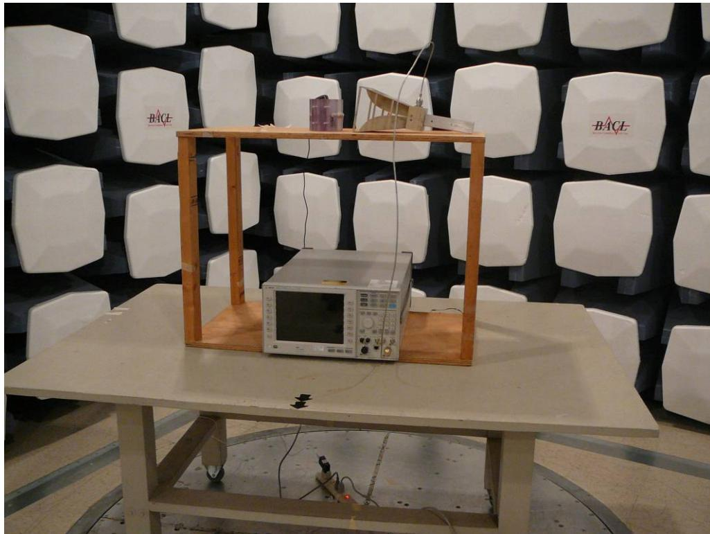
**Transmitter Radiated Emissions (Above 1 GHz) – Back View**
