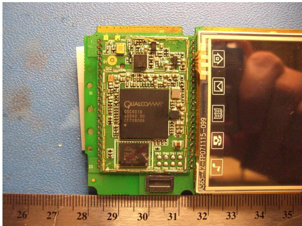
**RF Board with Shield on – Front View**
