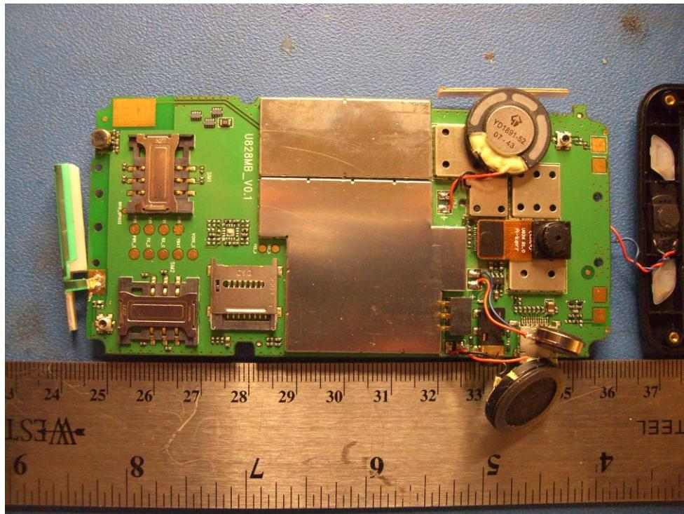
**RF Board with Shield off – Front View**
