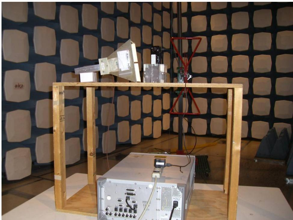
**Radiated Emissions (Above 1 GHz) – Back View**
