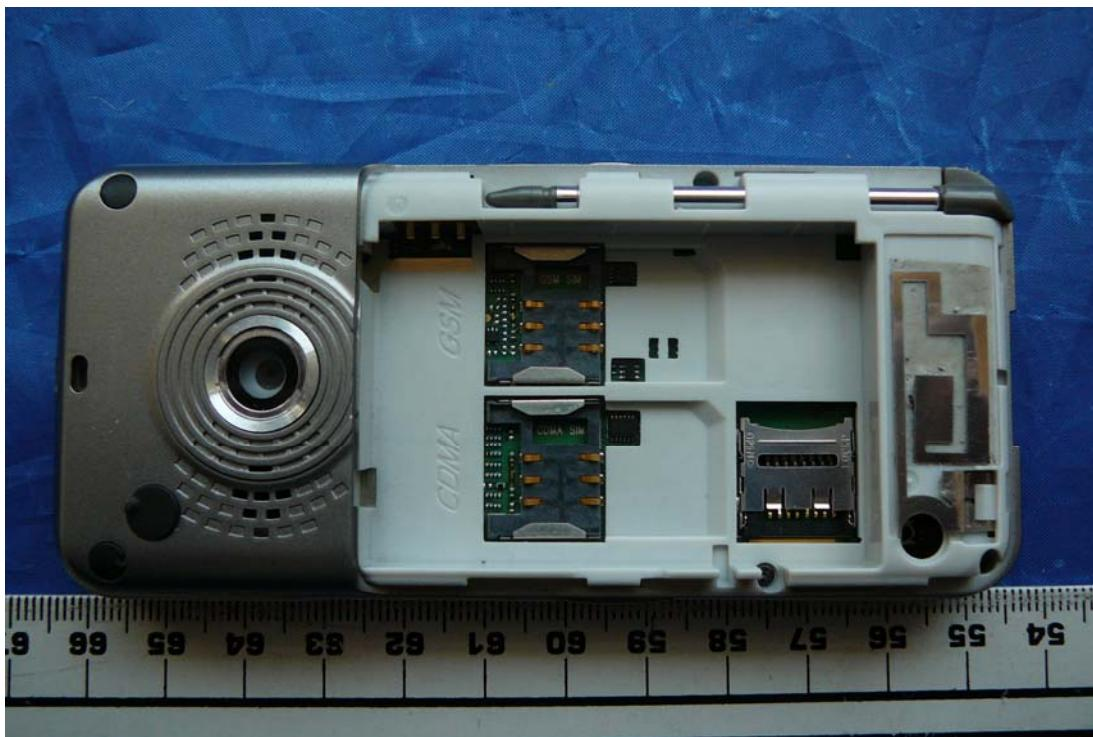
**EUT Internal – Main board Top Component View (1): With LCD and RF Shield**
