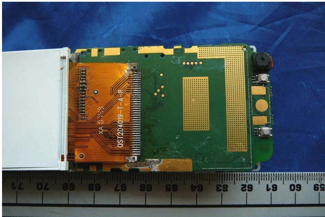
**EUT Internal – Main board Top Component View (4): RF Section close up view**
