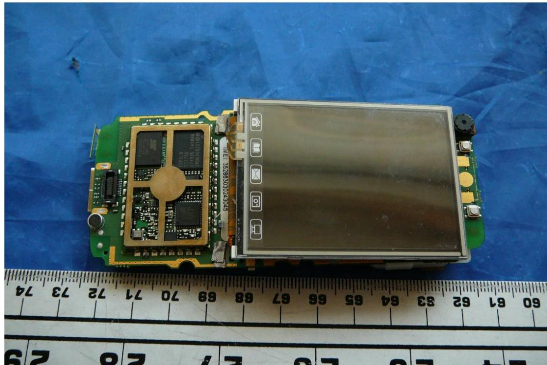
**EUT Internal – Main board Top Component View (3): Without LCD**
