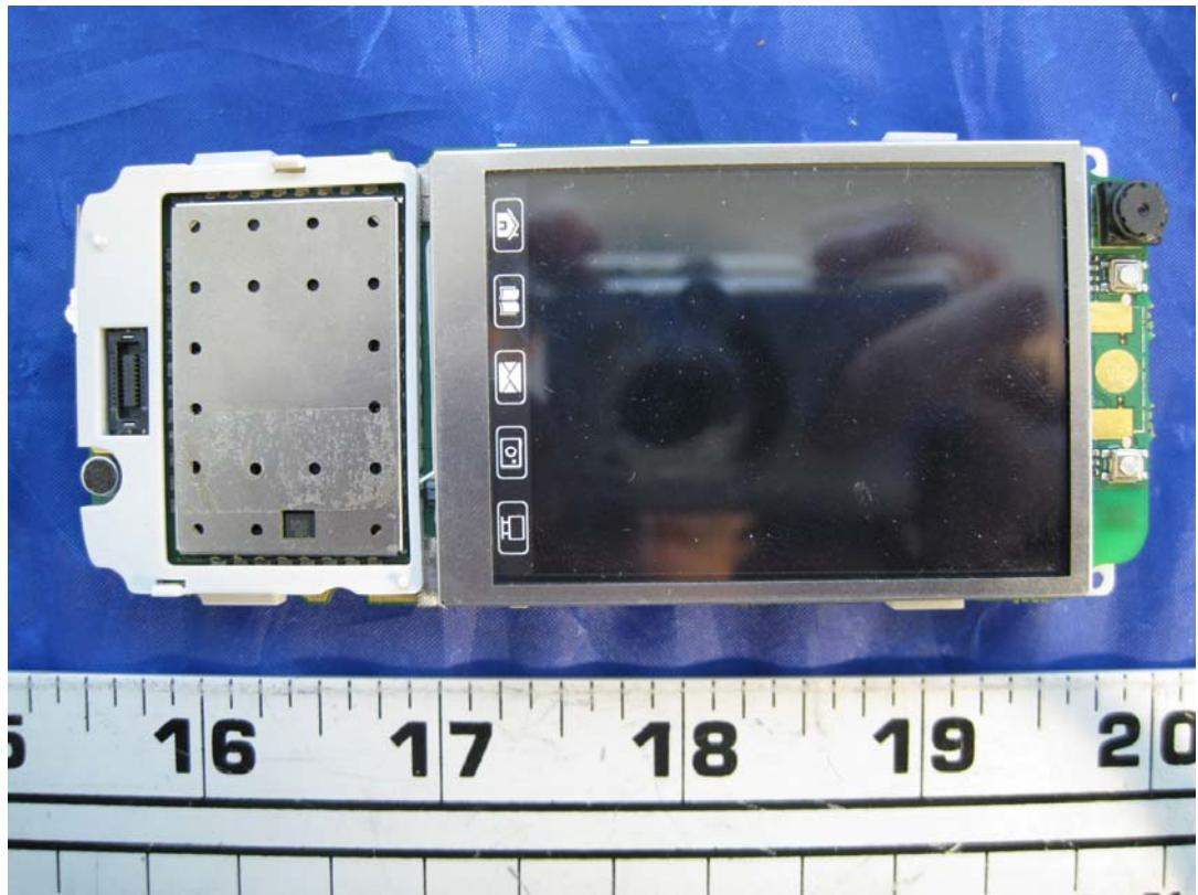
**EUT Internal – Main board Top Component View (2): Without RF Shield**
