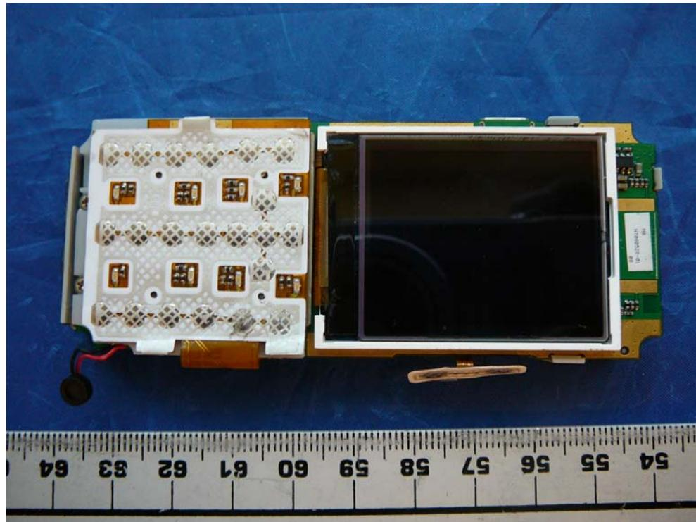
**EUT Internal – Main board Top Component View (2): Without Keyboard**
