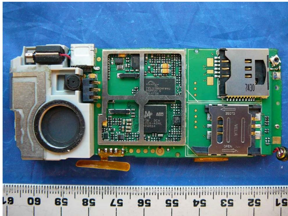
**EUT Internal – Main board back Component View (3): Near view**
