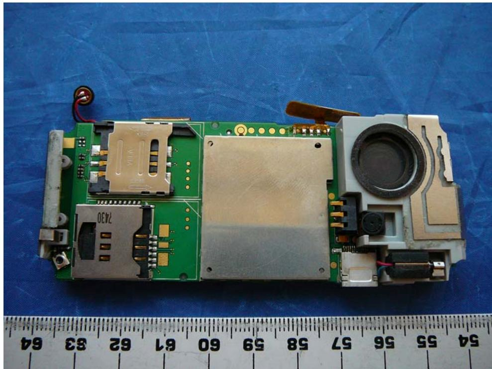
**EUT Internal – Main board back Component View (2): Without RF shielding**
