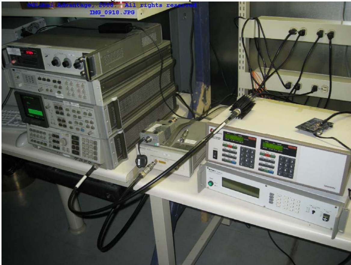
Figure 6 – Conducted power emissions
