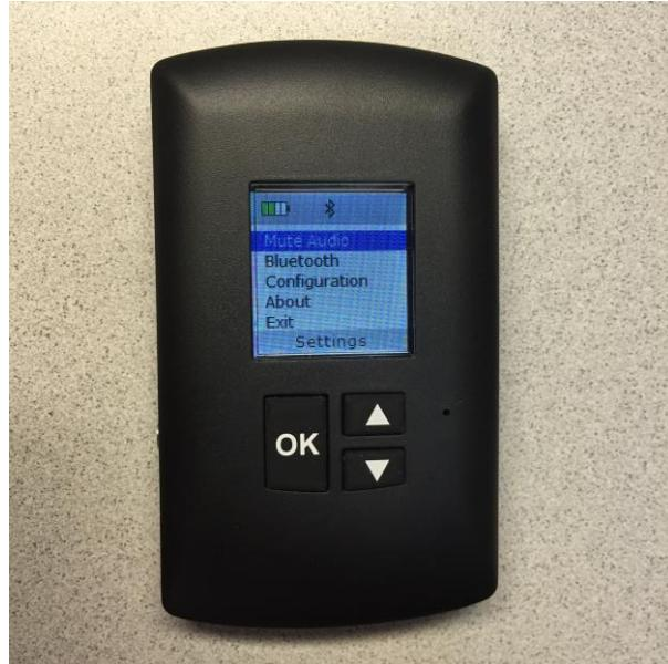
Selecting "About" brings up the logo and firmware version, with an arrow at the bottom of the screen indicating that more information is available for viewing, by scrolling downward:
