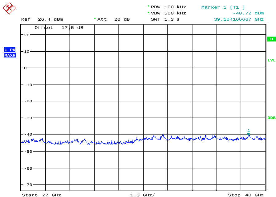
Plot 21: TX mode, lowest channel, 27 GHz to 40 GHz
