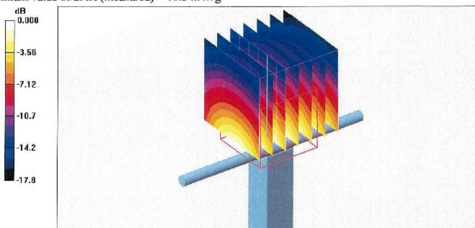
**Impedance Measurement Plot for Head TSL**
