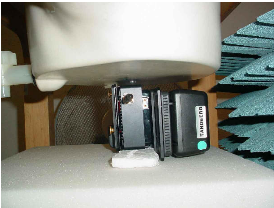
Photo 8: Test position body worn left side with distance 25 mm from antenna to SAM
