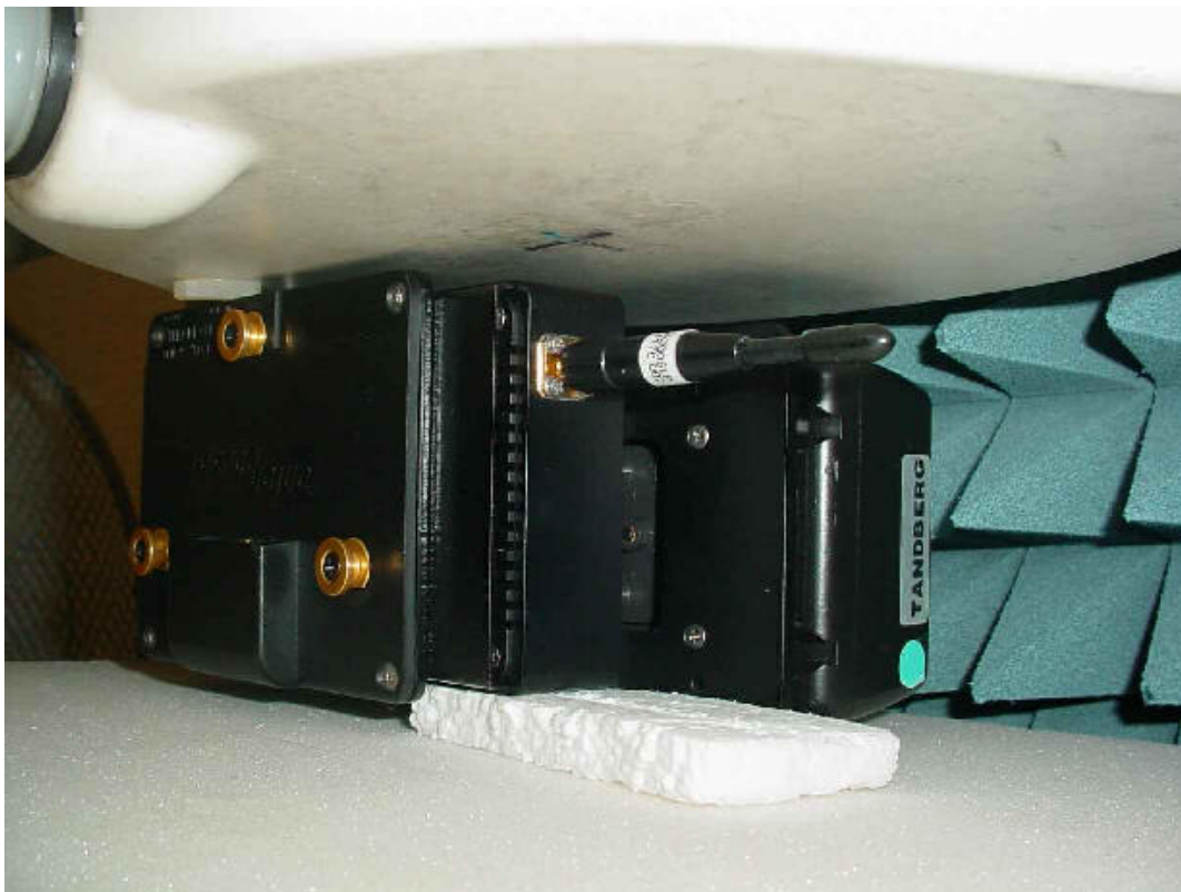
Photo 8: Test position body worn left side with distance 25 mm from antenna to SAM
