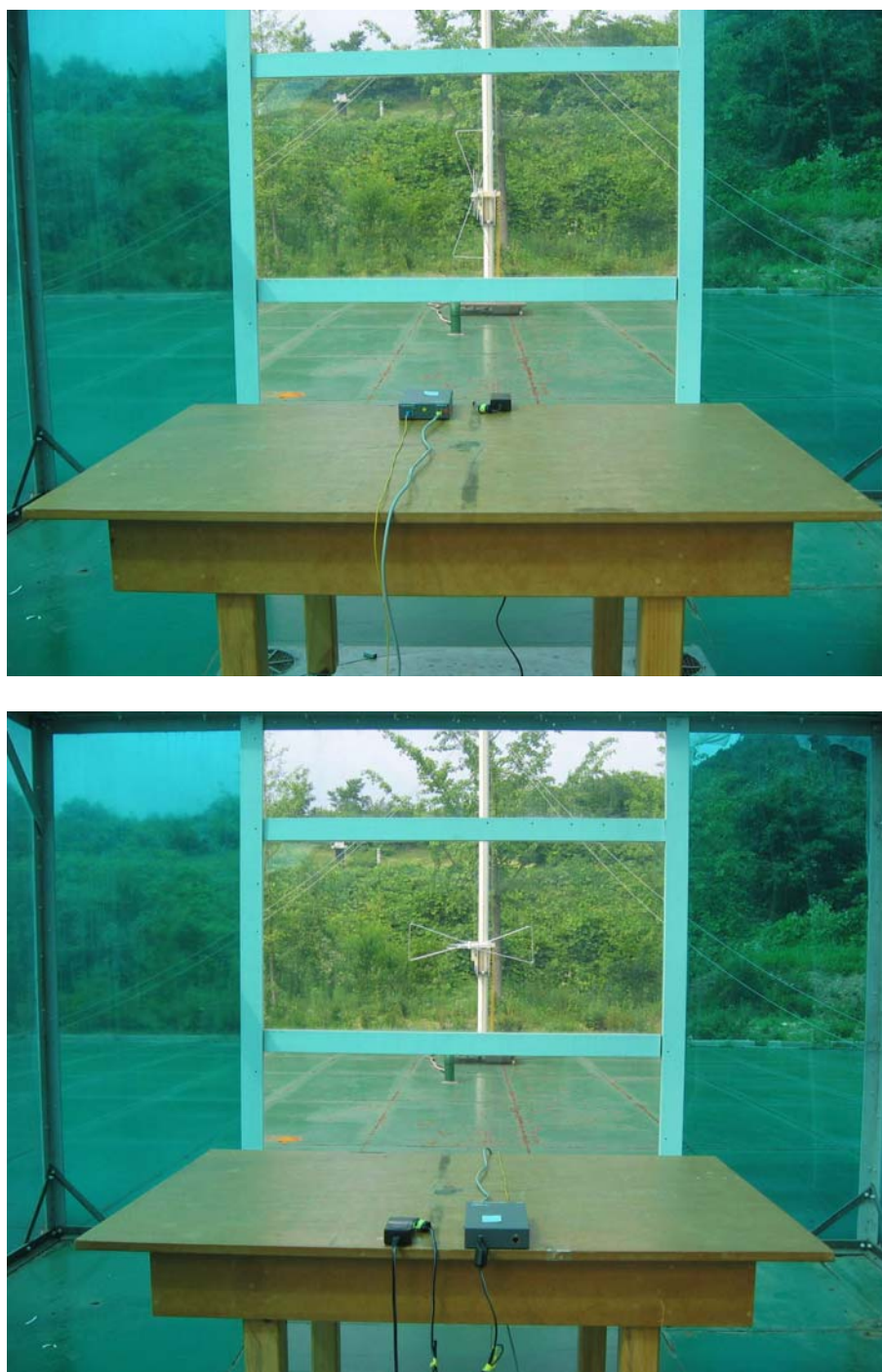
Figure 4. Photo of Radiated emission test setup
