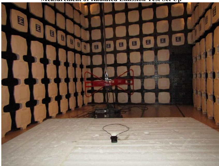
Measurement of Radiated Emission Test Set Up
