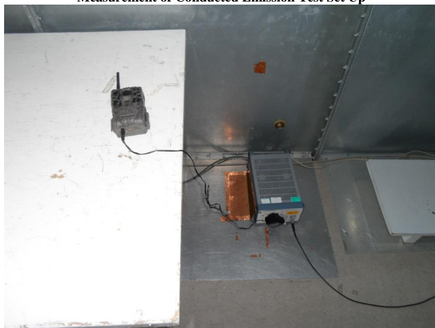
Measurement of Conducted Emission Test Set Up
