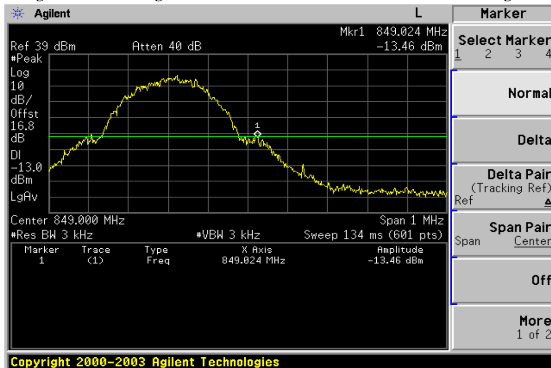
Figure 8-5: Band edge emission at antenna terminals – GSM Channel Highest
