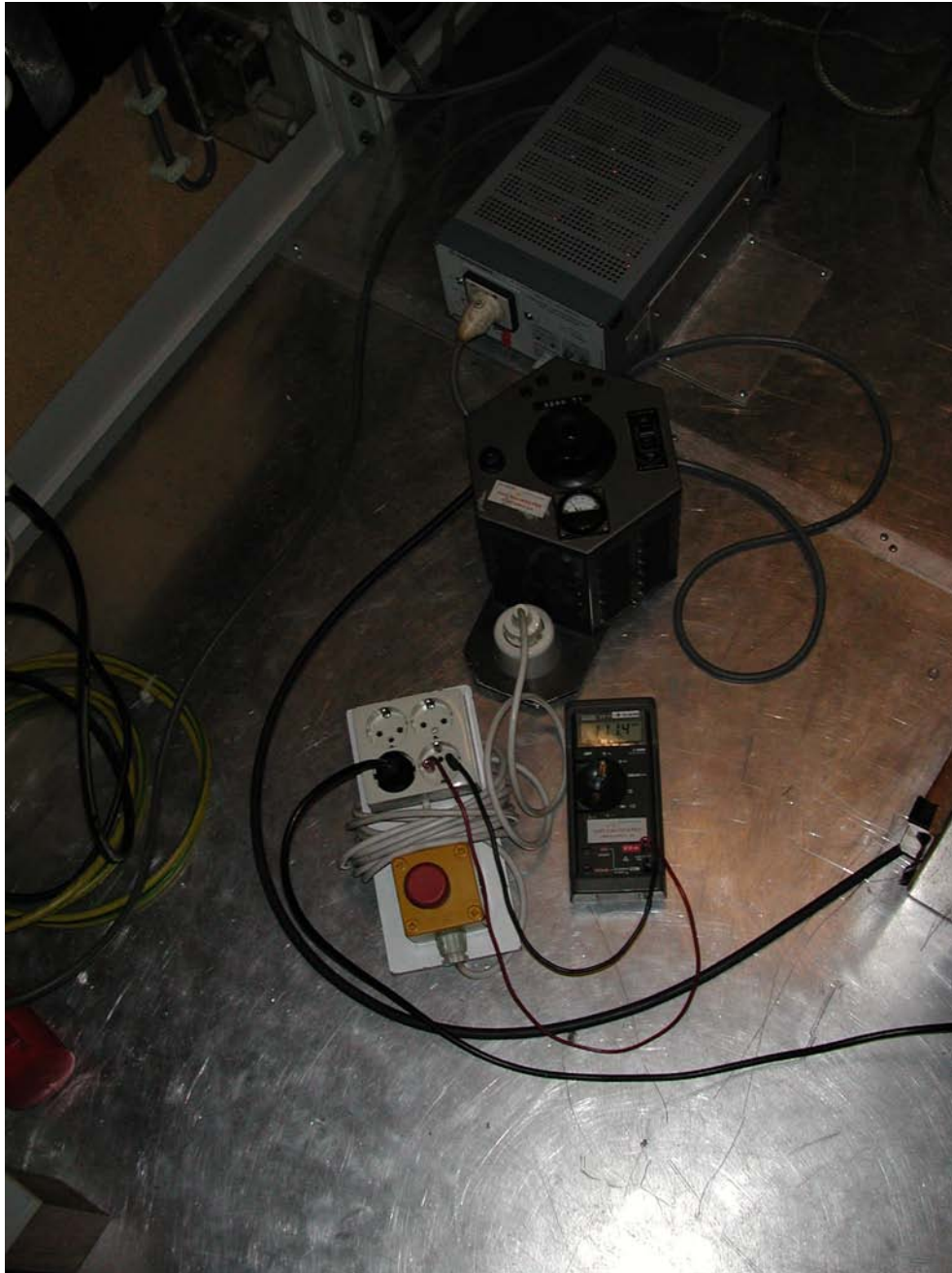
Photograph 5: Test setup conducted emission, measurement equipment
