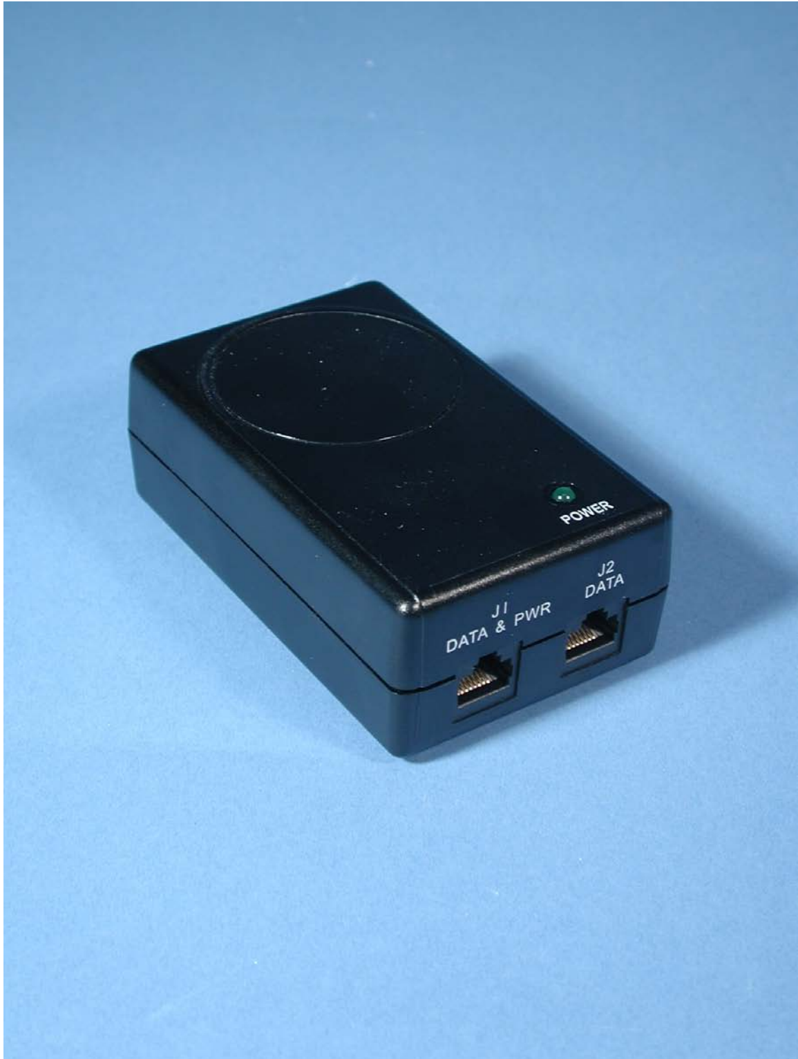
Photograph 9: Power over Ethernet hub
