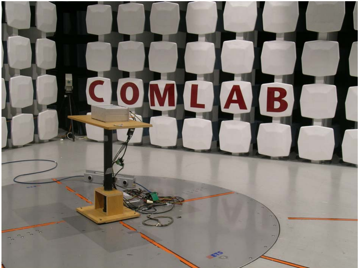
Test set-up for Radiated measurements
