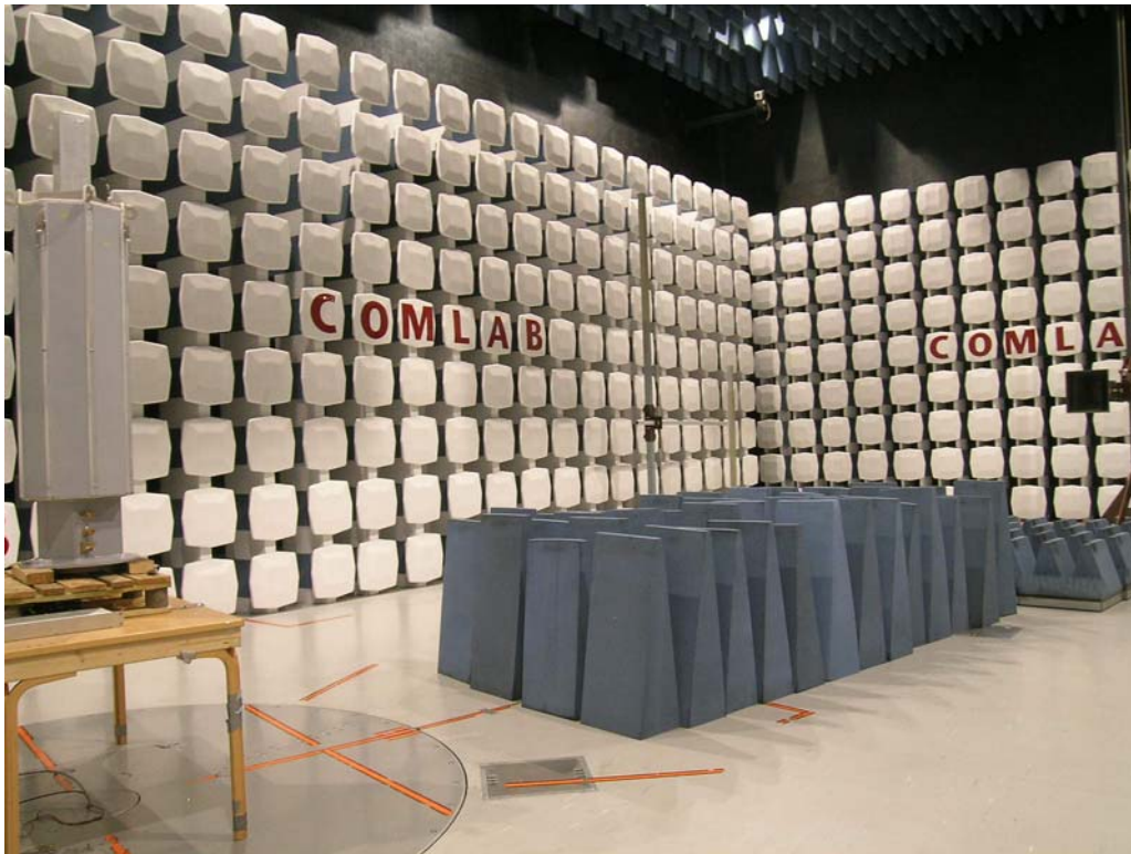
Test set-up for Radiated measurements
