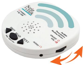
To **shut off** the unit, turn the thumbwheel counter-clockwise until you hear a click.
