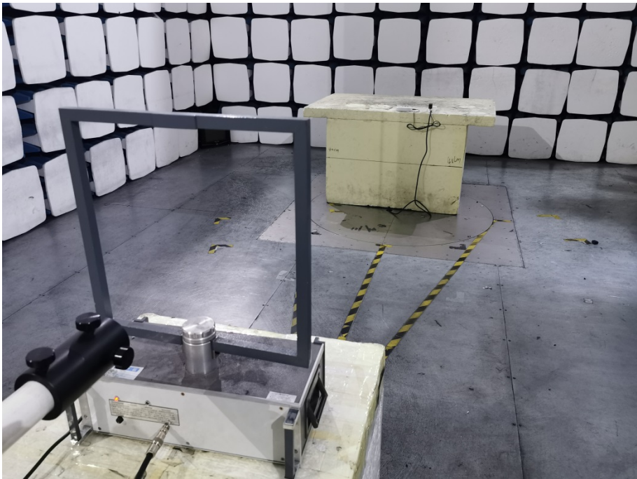
Radiation Emission Test Setup (Below 30MHz)
