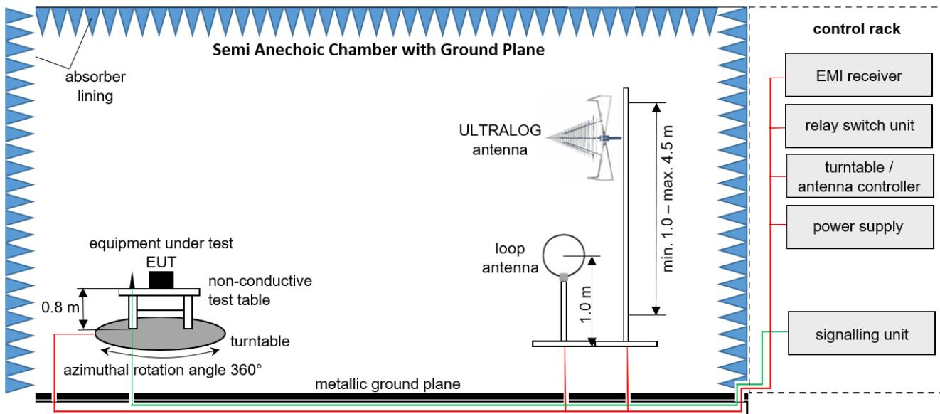
Measurement distance: ULTRALOG antenna at 3 m; loop antenna at 3 m
