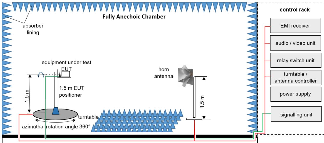
Measurement distance: horn antenna at 3 m
