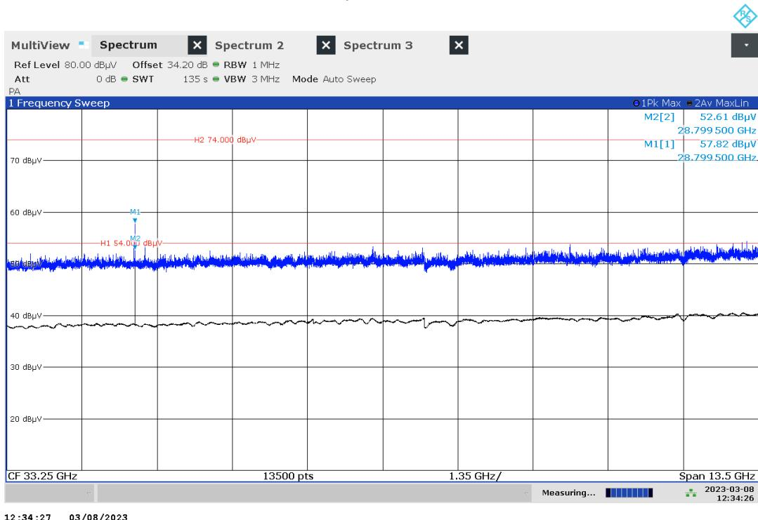
Plot no. 66: radiated emissions zoomed in on 28.8 GHz emission, polarization vertical / horizontal, DUT 1 normal
