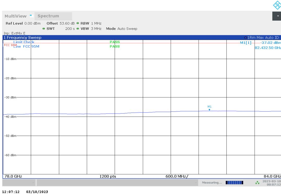
Plot no. 72: radiated emissions 84 GHz – 110 GHz, polarization vertical / horizontal, DUT 1 normal
