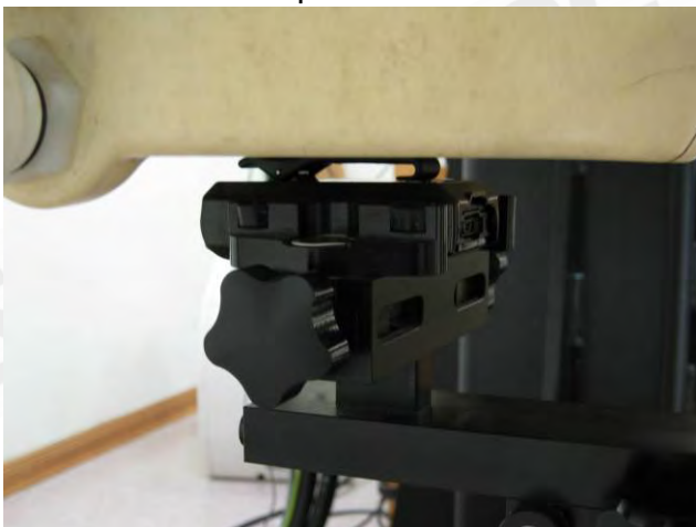
Fig.4 Put the EUT into holster and back side of EUT is paralleled with flat phantom, holster is paralleled and contacted with flat phantom.
