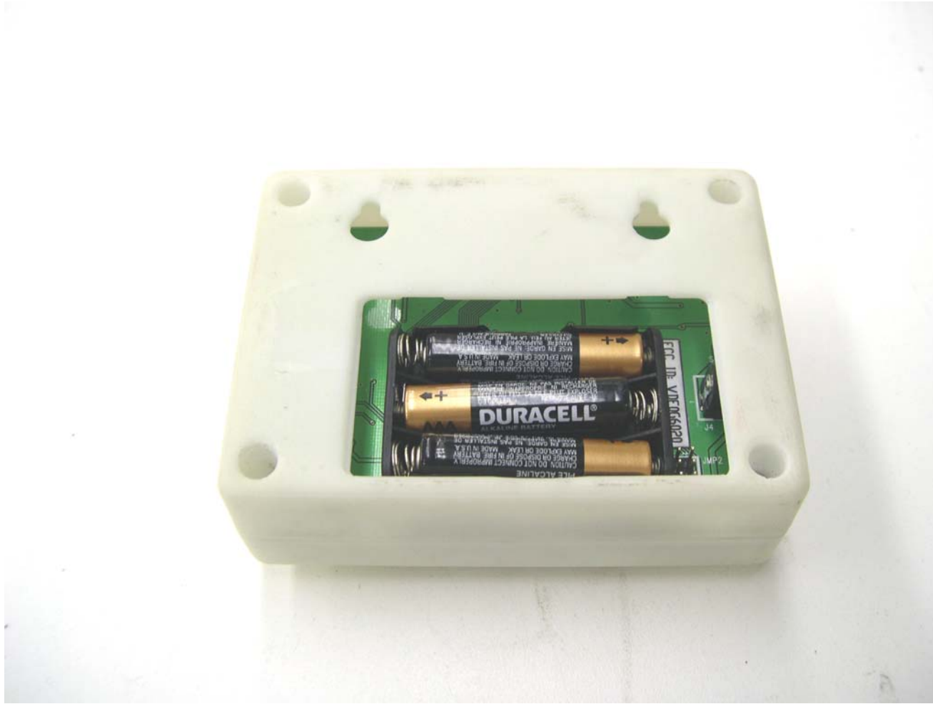
0G6020: Rear view of case showing battery compartment.
