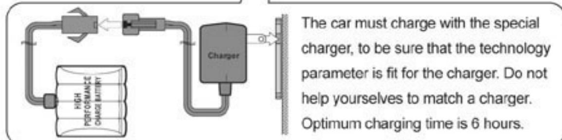
The car must charge with the special charger, to be sure that the technology parameter is fit for the charger. Do not help yourselves to match a charger. Optimum charging time is 6 hours.
