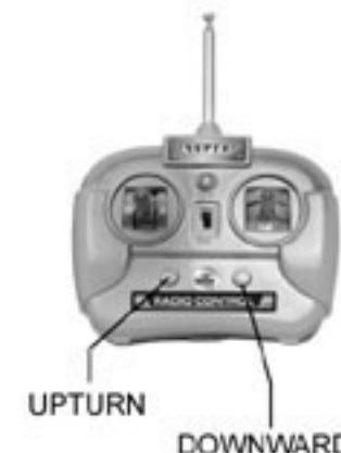
4. Press the key to control the scraper up and down.
