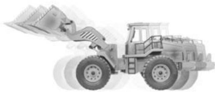
3. Turn the lever forward and backward, to control the scraper truck forward and backward.
