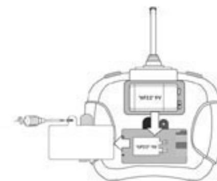
1. Open the cover put in the 9V battery, turn the switch to "ON".
