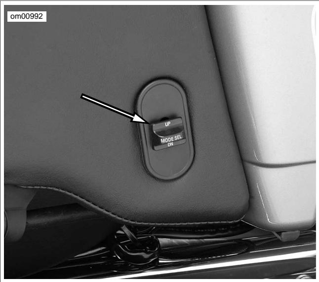
**Figure 30. Passenger UP/MODE SEL/DN Switch:
