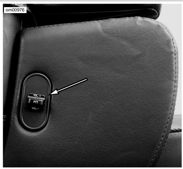
Figure 31. Passenger PTT/+VOL/- Switch: FLHTCUSE3
