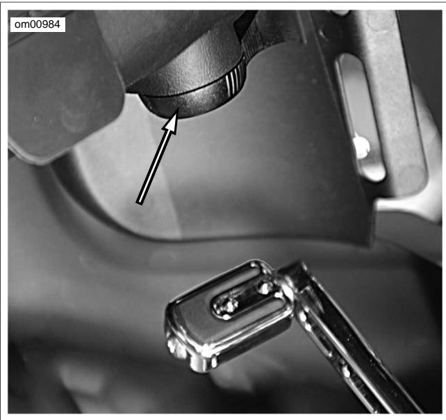
**Figure 18. Fairing Lower Vent Control: FLHTCUSE3**
