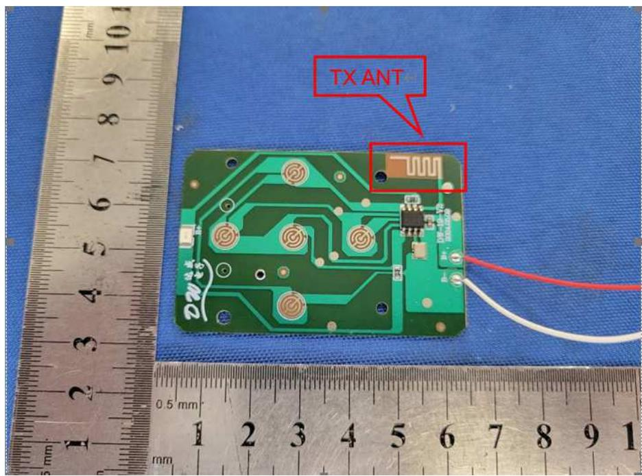
Antenna Type: PCB Antenna
