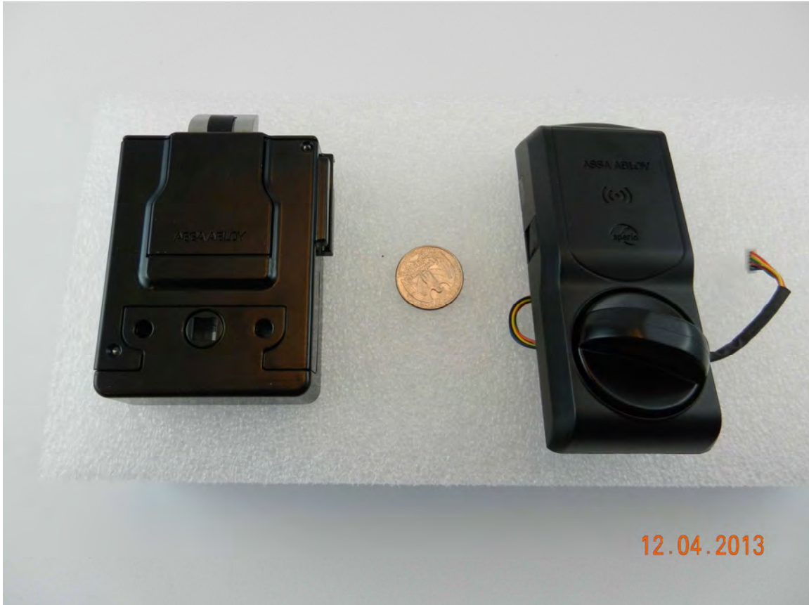
Placed next to a quarter for scale – lockbody on left, reader on right
