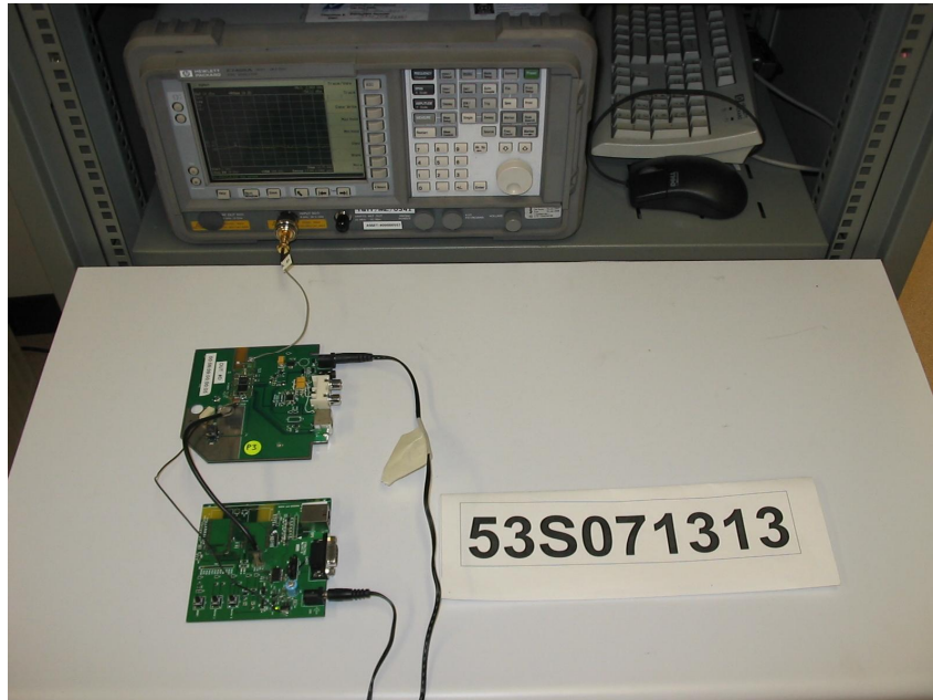
Average Frequency Dwell Time Test Setup
