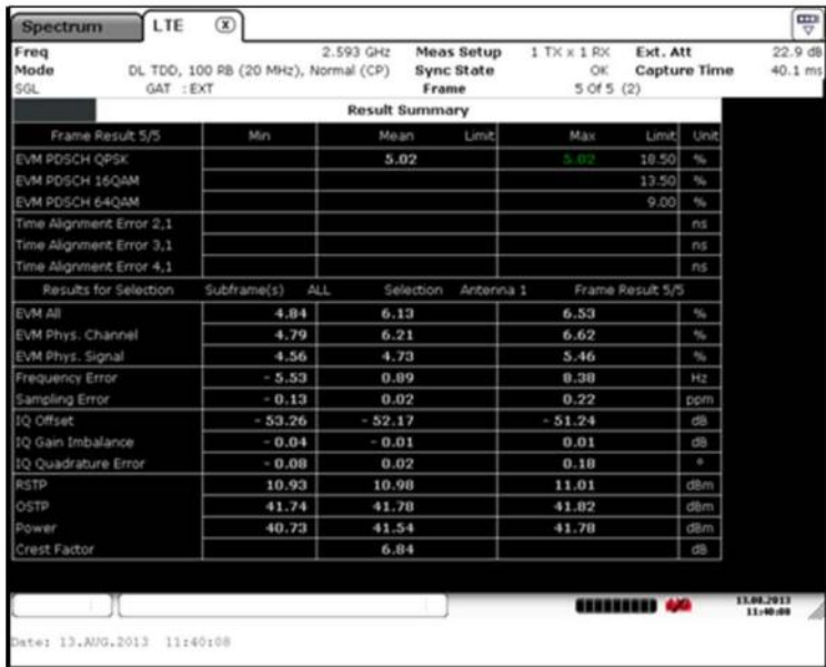
Figure 60 I/Q constellation table with I/Q error – QPSK (2593.0 MHz) (20MHz Channel BW)
