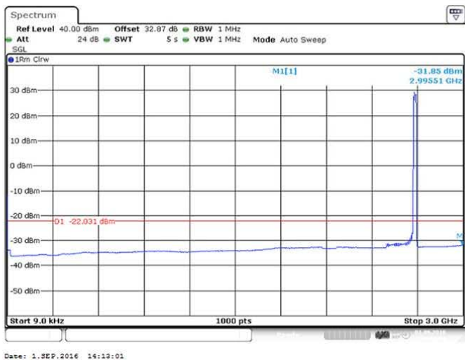
Figure 45 Spurious Emissions (9kHz – 3GHz) – 16QAM (2593.0 MHz) (20MHz Channel BW)
