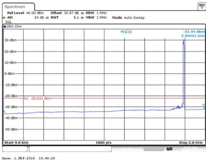
Figure 125 Spurious Emissions (9kHz – 3GHz) – 64QAM (2593.0 MHz) (20MHz Channel BW)
