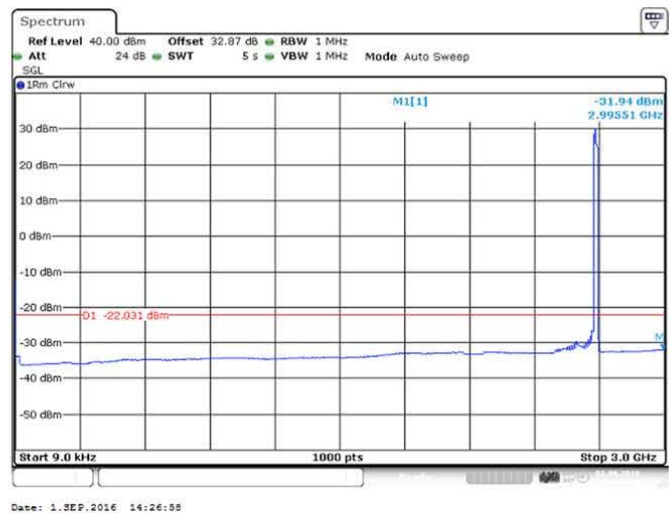
Figure 61 Spurious Emissions (9kHz – 3GHz) – QPSK (2593.0 MHz) (20MHz Channel BW)
