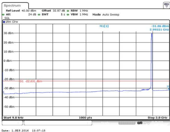
Figure 132 Spurious Emissions (9kHz – 3GHz) - QPSK (2593.0 MHz) (20MHz Channel BW)
