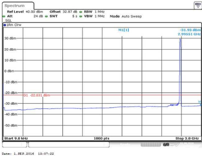
Figure 97 Spurious Emissions (9kHz – 3GHz) - QPSK (2593.0 MHz) (20MHz Channel BW)
