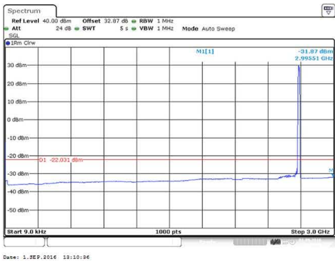
Figure 101 Spurious Emissions (9kHz – 3GHz) – 64QAM (2593.0 MHz) (20MHz Channel BW)
