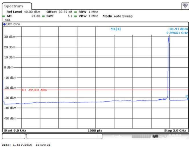
Figure 105 Spurious Emissions (9kHz – 3GHz) – 16QAM (2593.0 MHz) (20MHz Channel BW)
