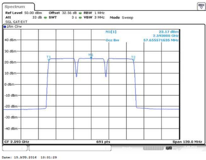
Figure 62 Occupied Bandwidth–QPSK (2573/ 2593/ 2613 MHz) (3 X 20 MHz Channel BW)
