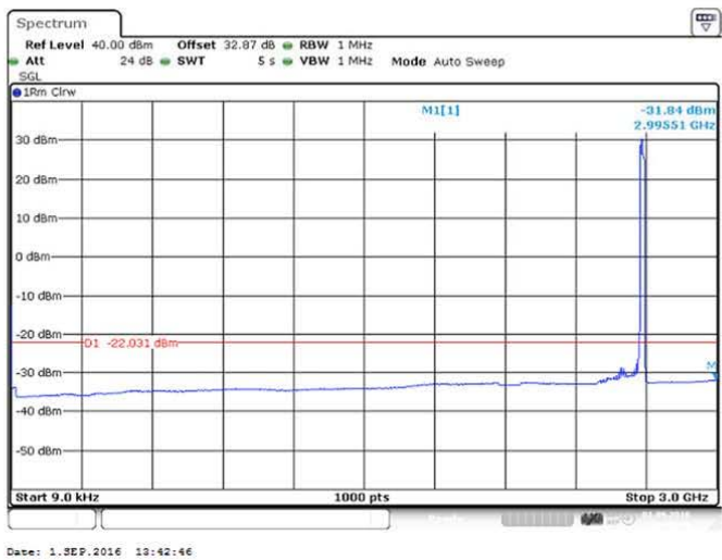
Figure 121 Spurious Emissions (9kHz – 3GHz) - QPSK (2593.0 MHz) (20MHz Channel BW)
