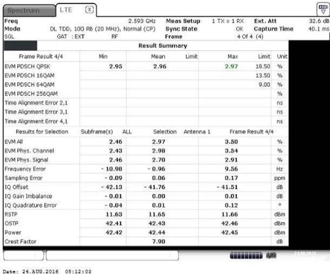
Figure 6 I/Q constellation table with I/Q error – QPSK (2593.0 MHz) (20MHz Channel BW)
