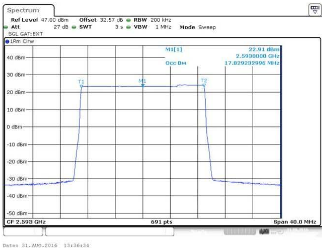
Figure 20 Occupied Bandwidth – QPSK (2593.0 MHz) (20MHz Channel BW)
