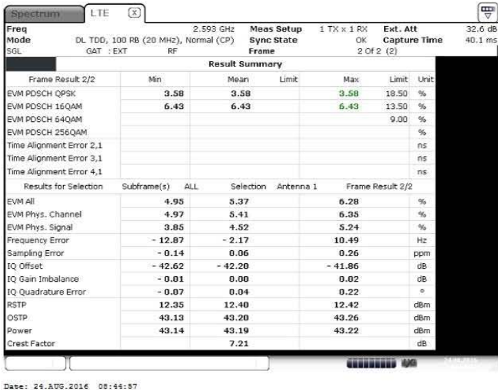
Figure 10 I/Q constellation table with I/Q error – 16QAM (2593.0 MHz) (20MHz Channel BW)
