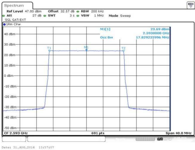
Figure 24 Occupied Bandwidth – 64QAM (2593.0 MHz) (20MHz Channel BW)
