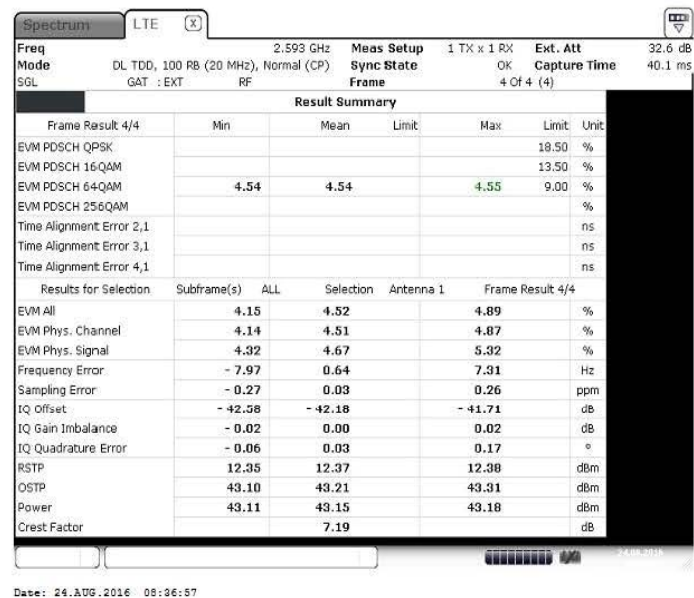
Figure 8 I/Q constellation table with I/Q error – 64QAM (2593.0 MHz) (20MHz Channel BW)
