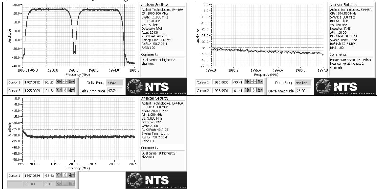
**Transmitter Antenna Port Conducted Spurious Emissions**
