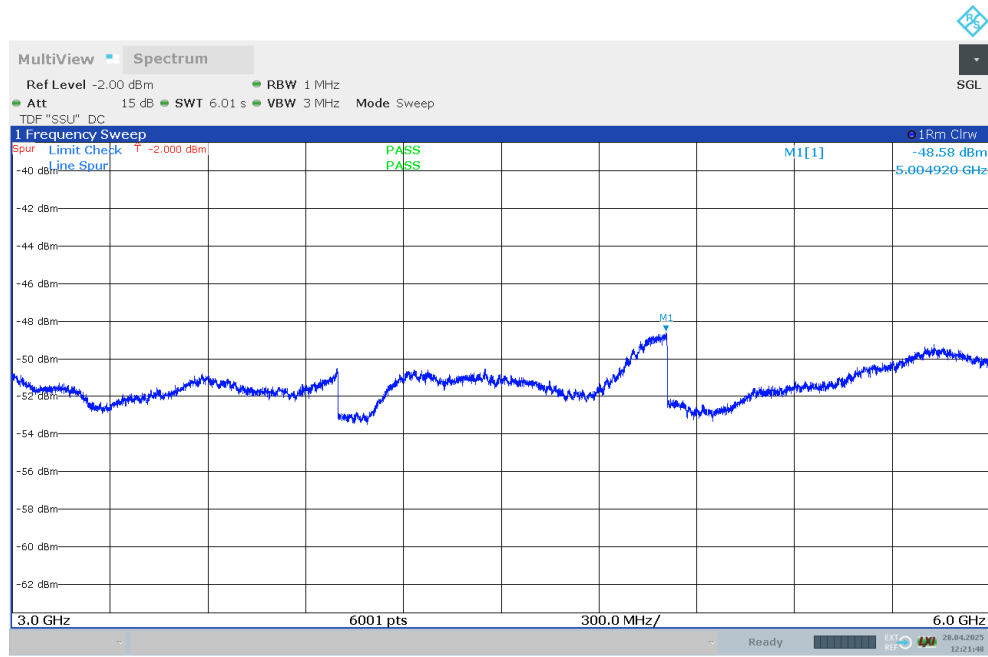
Figure 36 Spurious Emissions (3GHz–6GHz) – 16QAM (1962.5 MHz) (LTE 5MHz Channel BW)
