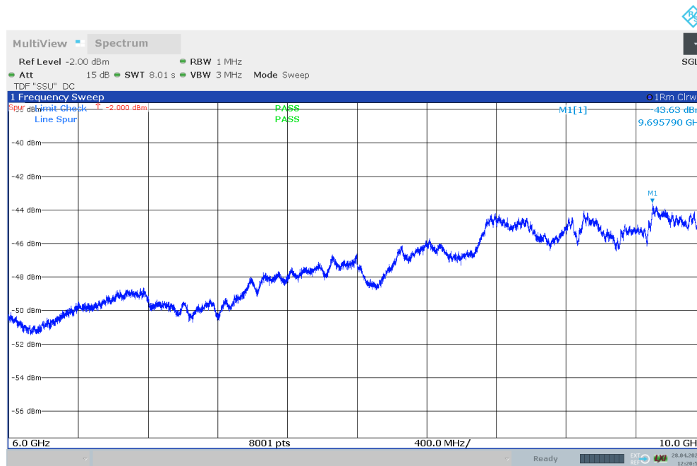
Figure 37 Spurious Emissions (6GHz–10GHz) – 16QAM (1962.5 MHz) (LTE 5MHz Channel BW)
