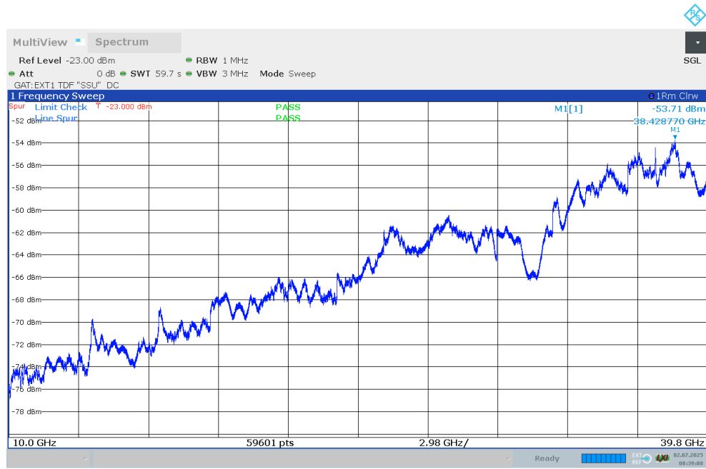
Figure 45 Spurious Emissions (10–39.8GHz) – 16QAM (3840 MHz) (NR10MHz Channel BW)
