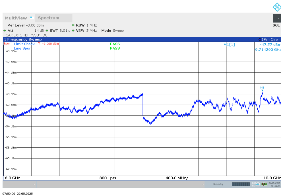
Figure 44 Spurious Emissions (6-10GHz) – 16QAM (3840 MHz) (NR10MHz Channel BW)
