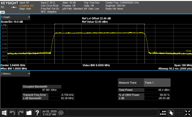
Port 1 90 MHz Channel Bandwidth 64QAM Modulation Middle Channel, 3840.00 MHz
