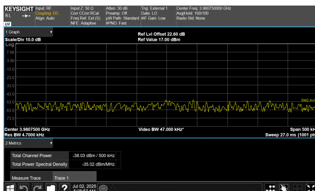
QPSK Modulation 50 MHz Channel Bandwidth High Channel, 3954.99 MHz 3980.5 MHz to 3981.0 MHz
