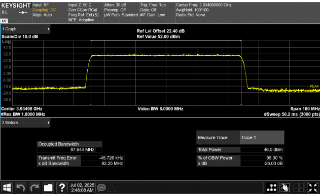
Port 1 90 MHz Channel Bandwidth QPSK Modulation High Channel, 3934.98 MHz
