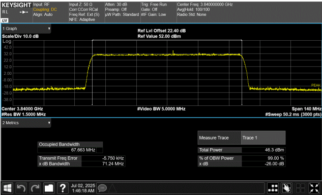
Port 1 70 MHz Channel Bandwidth QPSK Modulation Middle Channel, 3840.00 MHz
