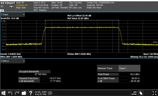
Port 1 70 MHz Channel Bandwidth 64QAM Modulation Middle Channel, 3840.00 MHz
