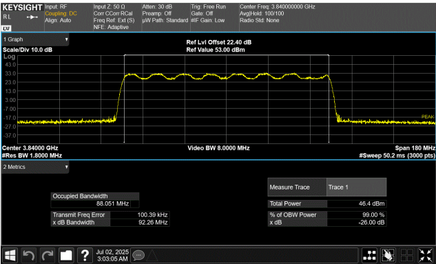
Port 1 90 MHz Channel Bandwidth 16QAM Modulation Middle Channel, 3840.00 MHz
