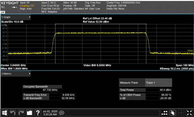
Port 1 90 MHz Channel Bandwidth 256QAM Modulation Middle Channel, 3840.00 MHz
