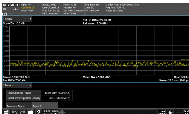
QPSK Modulation 50 MHz Channel Bandwidth Low Channel, 3725.01 MHz 3699.5 MHz to 3700.0 MHz
