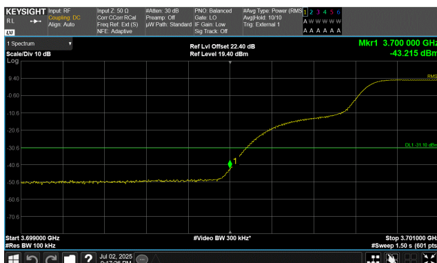
QPSK Modulation 10 MHz Channel Bandwidth Low Channel, 3705.00 MHz 3699.0 MHz to 3701.0 MHz
