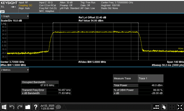
Port 1 70 MHz Channel Bandwidth QPSK Modulation Low Channel, 3735.00 MHz
