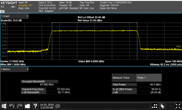
Port 1 90 MHz Channel Bandwidth QPSK Modulation Low Channel, 3745.02 MHz
