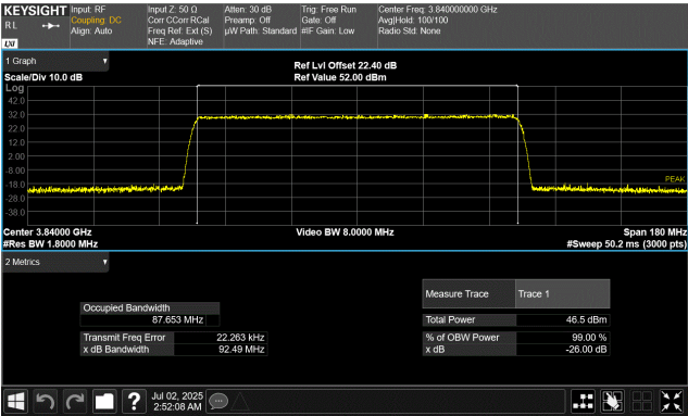
Port 1 90 MHz Channel Bandwidth QPSK Modulation Middle Channel, 3840.00 MHz
