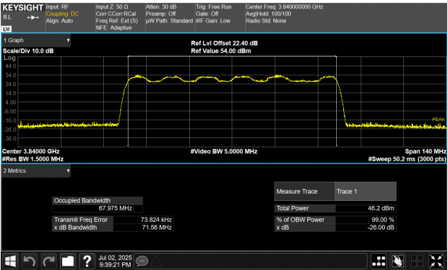
Port 1 70 MHz Channel Bandwidth 16QAM Modulation Middle Channel, 3840.00 MHz
