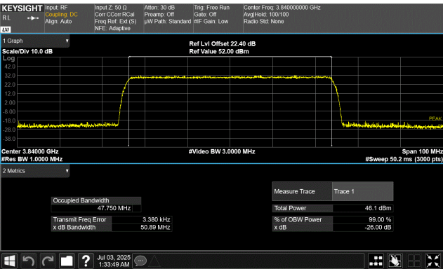
Port 1 50 MHz Channel Bandwidth 64QAM Modulation Middle Channel, 3840.00 MHz
