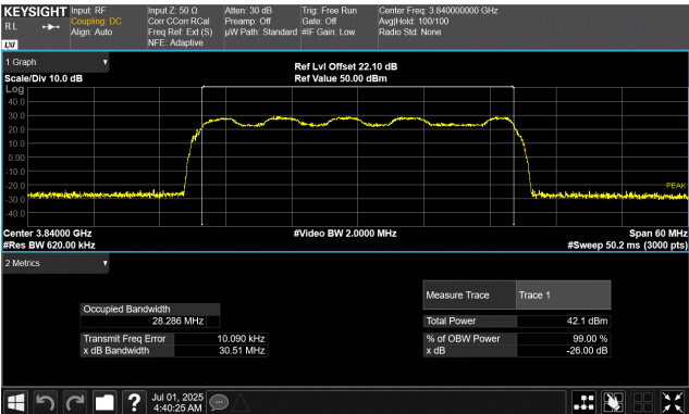
Port 1 30 MHz Channel Bandwidth 16QAM Modulation Middle Channel, 3840.00 MHz
