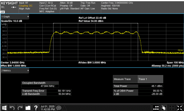
Port 1 50 MHz Channel Bandwidth 16QAM Modulation Middle Channel, 3840.00 MHz
