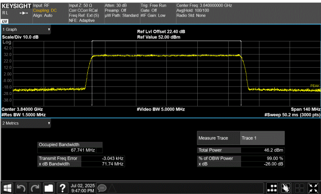
Port 1 70 MHz Channel Bandwidth 256QAM Modulation Middle Channel, 3840.00 MHz
