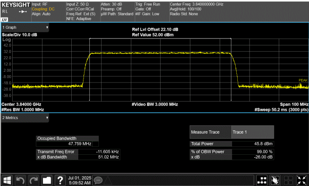
Port 1 50 MHz Channel Bandwidth QPSK Modulation Middle Channel, 3840.00 MHz
