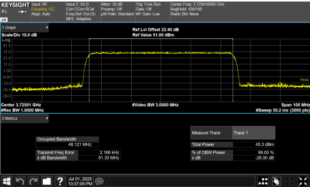
Port 1 50 MHz Channel Bandwidth QPSK Modulation Low Channel, 3725.01 MHz
