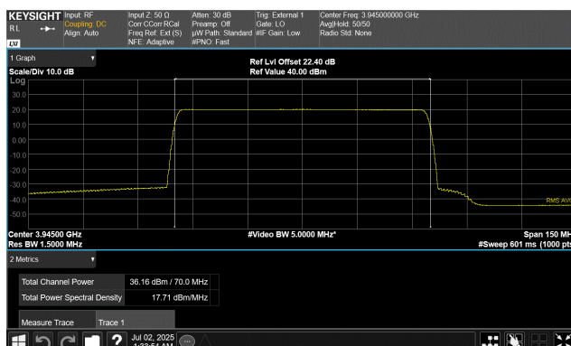
Port 1 70 MHz Channel Bandwidth QPSK Modulation High Channel, 3945.00 MHz
