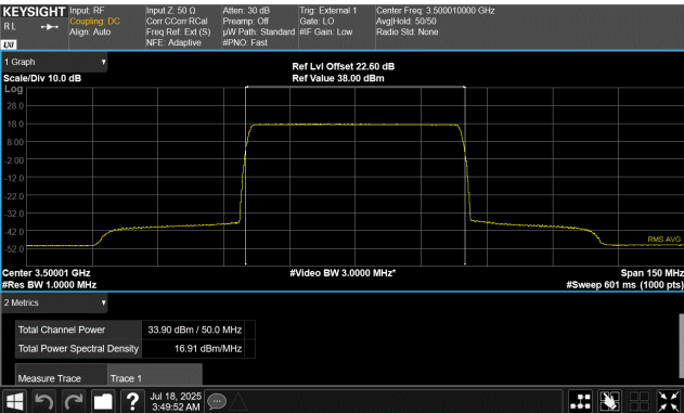
50 MHz Channel Bandwidth QPSK Modulation Middle Channel, 3500.01 MHz Port 63
