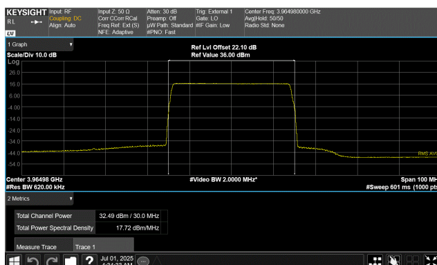
Port 1 30 MHz Channel Bandwidth QPSK Modulation High Channel, 3964.98 MHz
