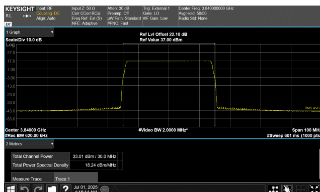
Port 1 30 MHz Channel Bandwidth QPSK Modulation Middle Channel, 3840.00 MHz
