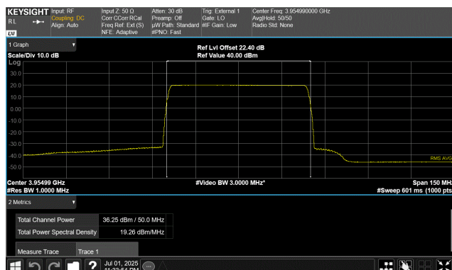
Port 1 50 MHz Channel Bandwidth QPSK Modulation High Channel, 3954.99 MHz
