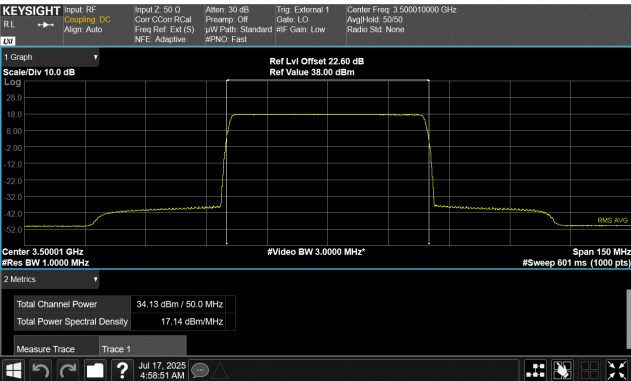
50 MHz Channel Bandwidth QPSK Modulation Middle Channel, 3500.01 MHz Port 3
