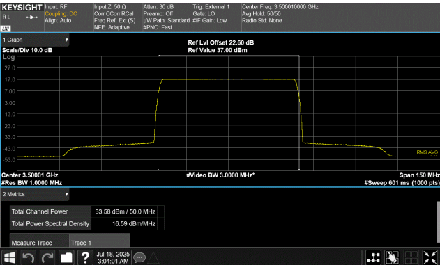
50 MHz Channel Bandwidth QPSK Modulation Middle Channel, 3500.01 MHz Port 27
