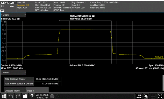
50 MHz Channel Bandwidth QPSK Modulation Middle Channel, 3500.01 MHz Port 34
