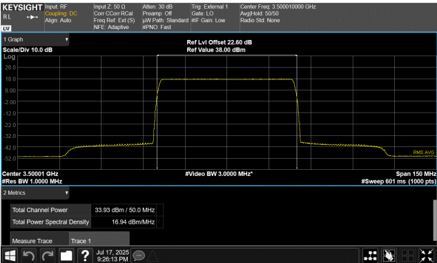
50 MHz Channel Bandwidth QPSK Modulation Middle Channel, 3500.01 MHz Port 4
