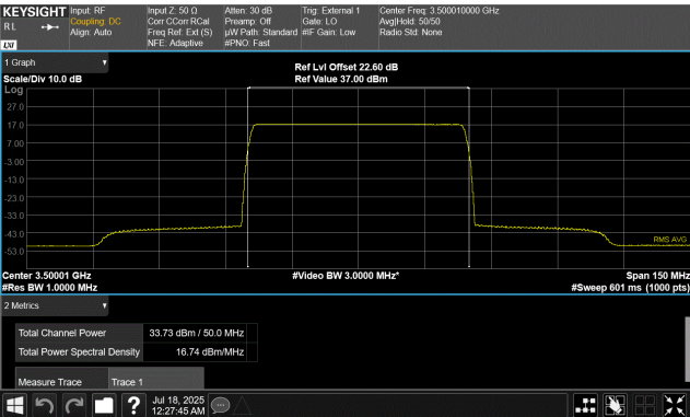
50 MHz Channel Bandwidth QPSK Modulation Middle Channel, 3500.01 MHz Port 51
