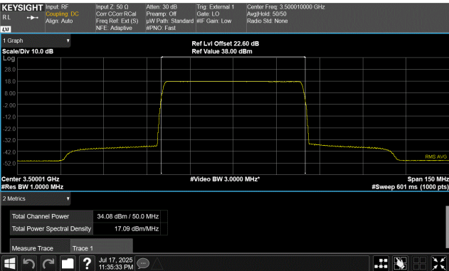
50 MHz Channel Bandwidth QPSK Modulation Middle Channel, 3500.01 MHz Port 15
