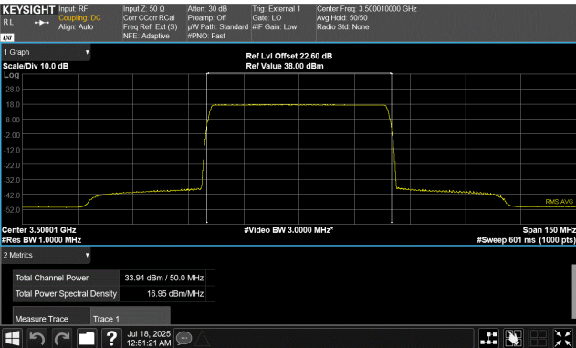
50 MHz Channel Bandwidth QPSK Modulation Middle Channel, 3500.01 MHz Port 21
