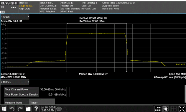
50 MHz Channel Bandwidth QPSK Modulation Middle Channel, 3500.01 MHz Port 57
