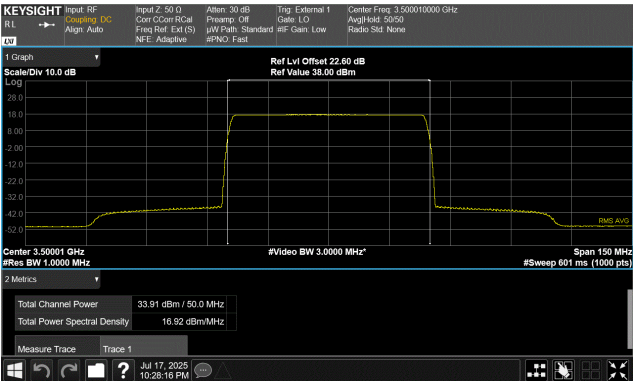
50 MHz Channel Bandwidth QPSK Modulation Middle Channel, 3500.01 MHz Port 10
