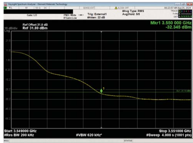
Port 1 20 MHz Channel Bandwidth QPSK Modulation High Channel, 3540.00 MHz
