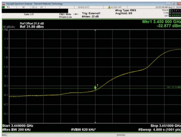
Port 1 QPSK Modulation Test Case 1
