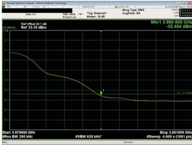
Port 1 QPSK Modulation Test Case 1
