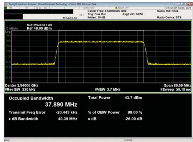
Port 1 40 MHz Channel Bandwidth QPSK Modulation Mid Channel, 3840.00 MHz
