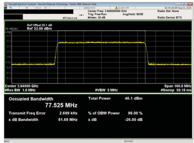
Port 1 80 MHz Channel Bandwidth QPSK Modulation Mid Channel, 3840.00 MHz
