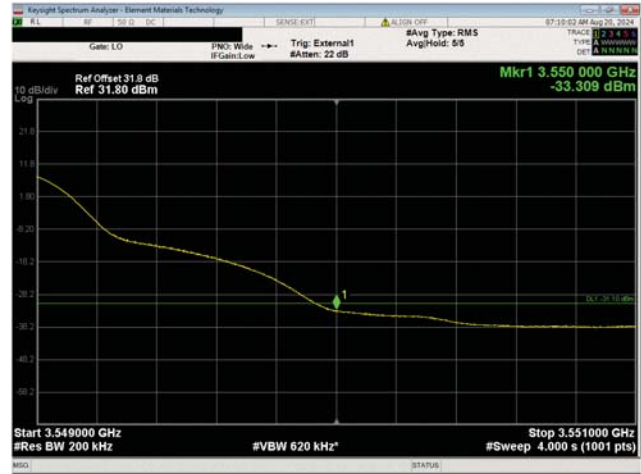
Port 1 30 MHz Channel Bandwidth QPSK Modulation High Channel, 3534.99 MHz
