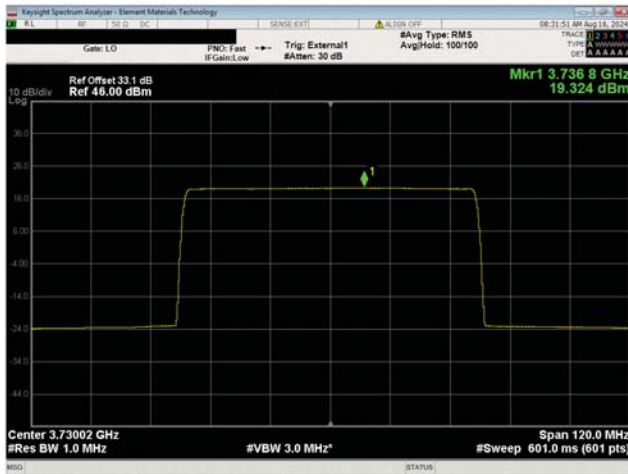
Port 1 60 MHz Channel Bandwidth QPSK Modulation Low Channel, 3730.02 MHz
