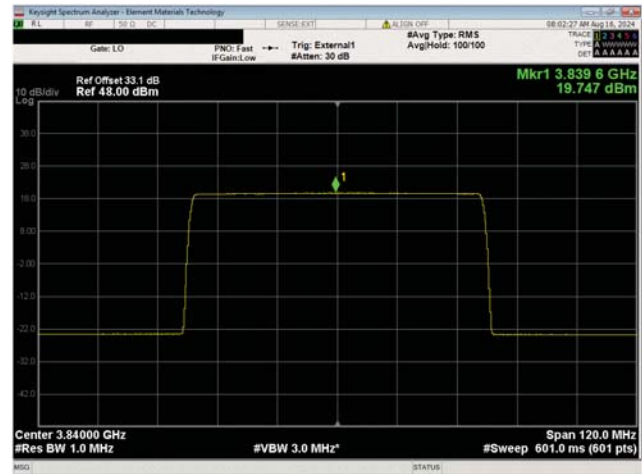
Port 1 60 MHz Channel Bandwidth QPSK Modulation Mid Channel, 3840.00 MHz
