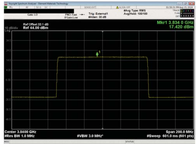
Port 1 100 MHz Channel Bandwidth 256QAM Modulation Mid Channel, 3840.00 MHz
