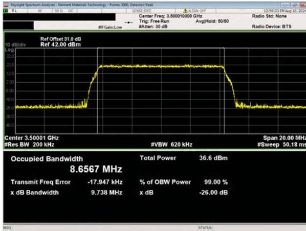
Port 1 10 MHz Channel Bandwidth 64QAM Modulation Mid Channel, 3500.01 MHz
