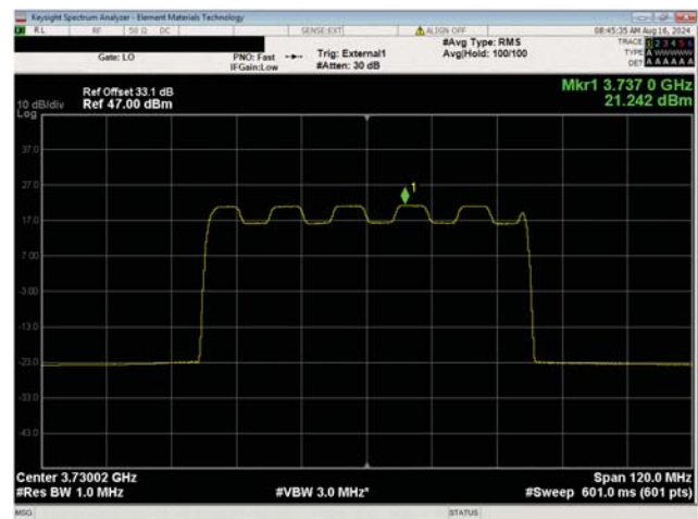
Port 1 60 MHz Channel Bandwidth 16QAM Modulation Low Channel, 3730.02 MHz
