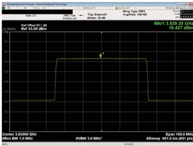
Port 1 80 MHz Channel Bandwidth 64QAM Modulation Mid Channel, 3840.00 MHz
