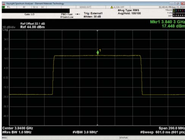
Port 1 100 MHz Channel Bandwidth 64QAM Modulation Mid Channel, 3840.00 MHz
