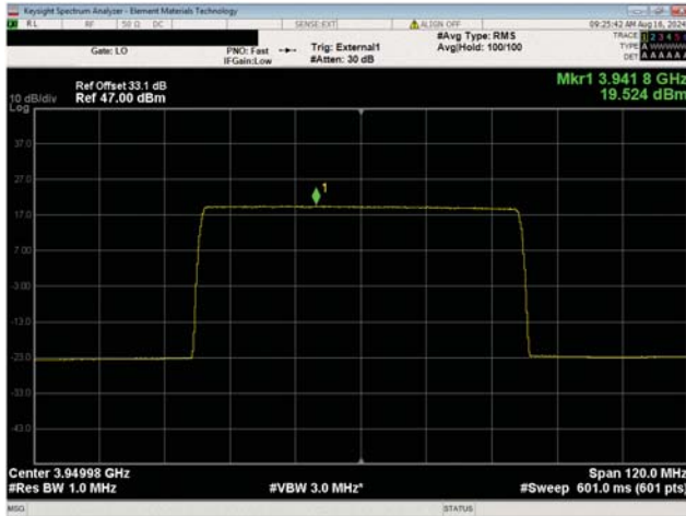
Port 1 60 MHz Channel Bandwidth 64QAM Modulation High Channel, 3949.98 MHz
