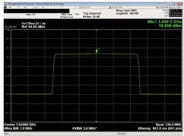
Port 1 60 MHz Channel Bandwidth 64QAM Modulation Mid Channel, 3840.00 MHz
