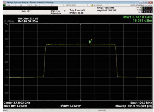
Port 1 60 MHz Channel Bandwidth 256QAM Modulation Low Channel, 3730.02 MHz
