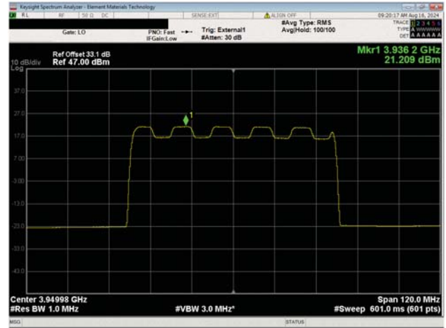
Port 1 60 MHz Channel Bandwidth 16QAM Modulation High Channel, 3949.98 MHz
