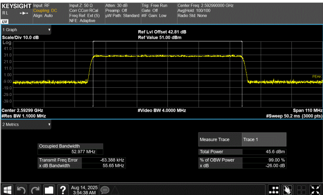
60 MHz Base Channel Bandwidth 55.0 MHz Slim Carrier Bandwidth 256QAM Modulation Middle Channel, 2529.99 MHz
