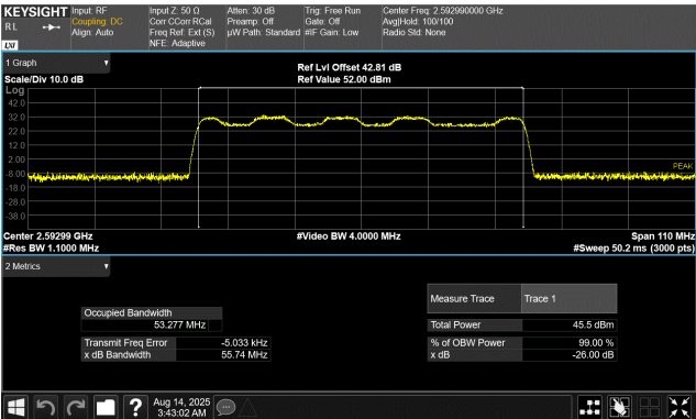
60 MHz Base Channel Bandwidth 55.0 MHz Slim Carrier Bandwidth 16QAM Modulation Middle Channel, 2529.99 MHz
