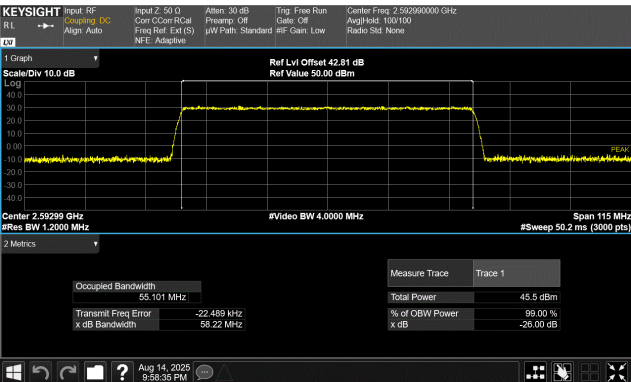
60 MHz Base Channel Bandwidth 57.5 MHz Slim Carrier Bandwidth 64QAM Modulation Middle Channel, 2592.99 MHz
