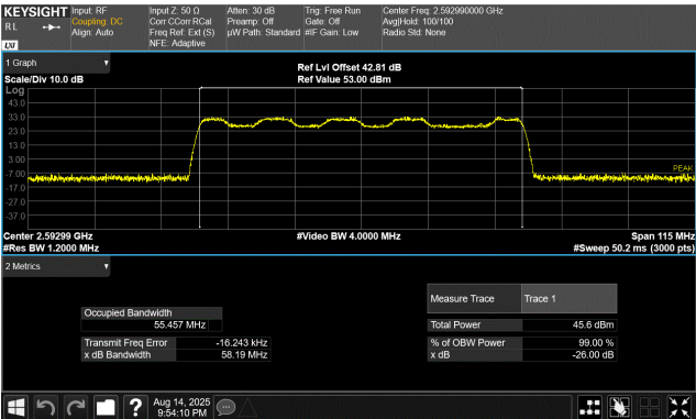
60 MHz Base Channel Bandwidth 57.5 MHz Slim Carrier Bandwidth 16QAM Modulation Middle Channel, 2592.99 MHz
