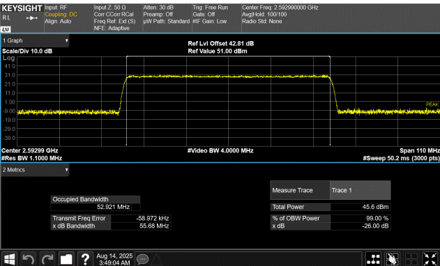
60 MHz Base Channel Bandwidth 55.0 MHz Slim Carrier Bandwidth 64QAM Modulation Middle Channel, 2529.99 MHz
