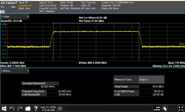
60 MHz Base Channel Bandwidth 55.0 MHz Slim Carrier Bandwidth QPSK Modulation Low Channel, 2526.00 MHz
