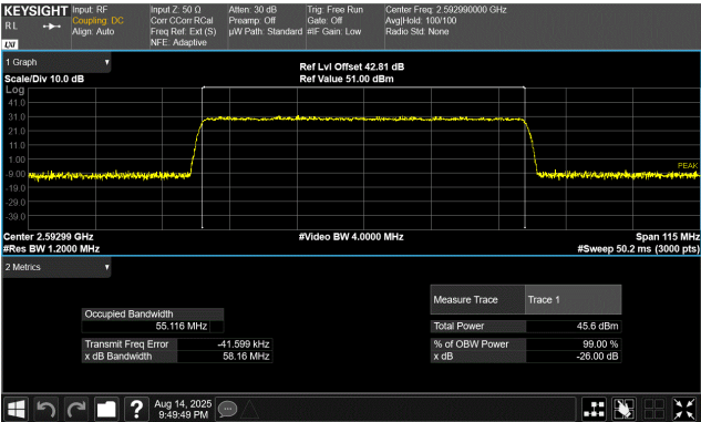
60 MHz Base Channel Bandwidth 57.5 MHz Slim Carrier Bandwidth QPSK Modulation Middle Channel, 2592.99 MHz
