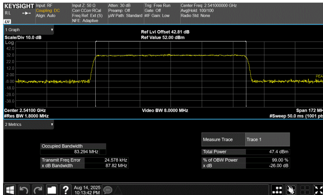
90 MHz Base Channel Bandwidth 86.0 MHz Slim Carrier Bandwidth QPSK Modulation Low Channel, 2541.00 MHz
