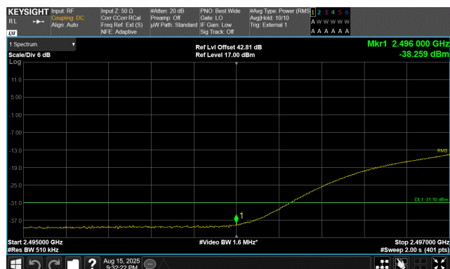
QPSK Modulation 49.0 MHz Slim Carrier Bandwidth Low Channel, 2521.02 MHz 2495 MHz - 2497 MHz
