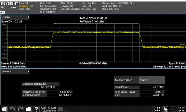
60 MHz Base Channel Bandwidth 57.5 MHz Slim Carrier Bandwidth 256QAM Modulation Middle Channel, 2592.99 MHz
