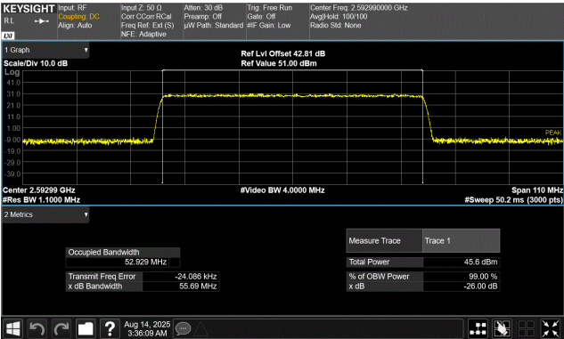
60 MHz Base Channel Bandwidth 55.0 MHz Slim Carrier Bandwidth QPSK Modulation Middle Channel, 2529.99 MHz
