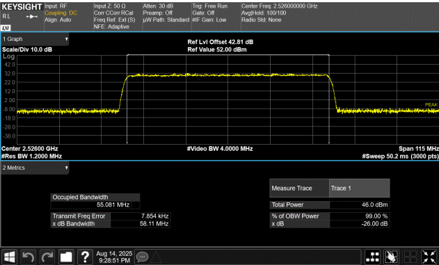
60 MHz Base Channel Bandwidth 57.5 MHz Slim Carrier Bandwidth QPSK Modulation Low Channel, 2562.00 MHz
