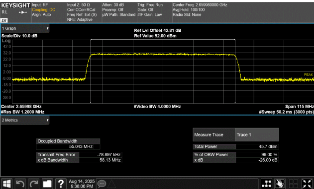
60 MHz Base Channel Bandwidth 57.5 MHz Slim Carrier Bandwidth QPSK Modulation High Channel, 2659.98 MHz
