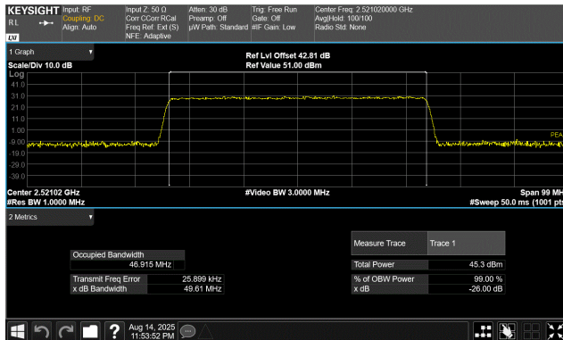
50 MHz Base Channel Bandwidth 49.5 MHz Slim Carrier Bandwidth QPSK Modulation Low Channel, 2521.02 MHz
