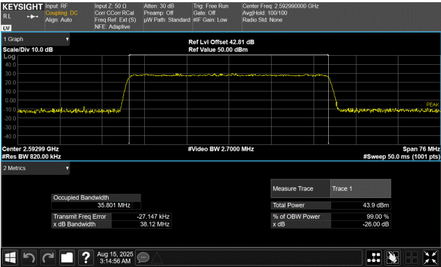
40 MHz Base Channel Bandwidth 38.0 MHz Slim Carrier Bandwidth QPSK Modulation Middle Channel, 2592.99 MHz
