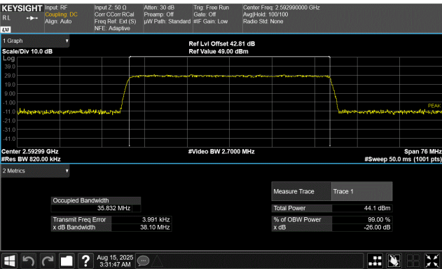
40 MHz Base Channel Bandwidth 38.0 MHz Slim Carrier Bandwidth 64QAM Modulation Middle Channel, 2592.99 MHz
