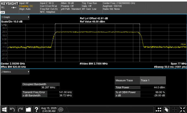
40 MHz Base Channel Bandwidth 38.5 MHz Slim Carrier Bandwidth 256QAM Modulation Middle Channel, 2592.99 MHz
