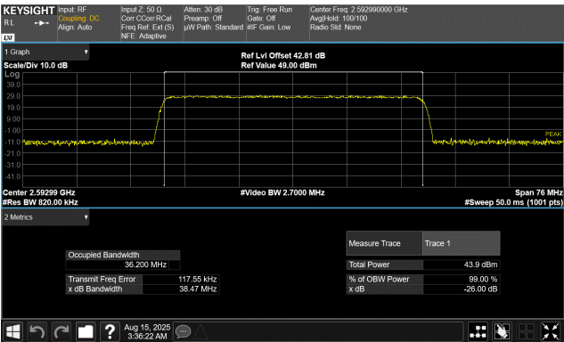
40 MHz Base Channel Bandwidth 38.0 MHz Slim Carrier Bandwidth 256QAM Modulation Middle Channel, 2592.99 MHz
