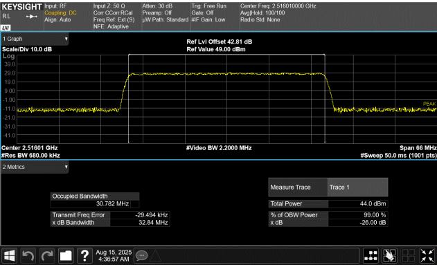
40 MHz Base Channel Bandwidth 33.0 MHz Slim Carrier Bandwidth QPSK Modulation Low Channel, 2516.01 MHz
