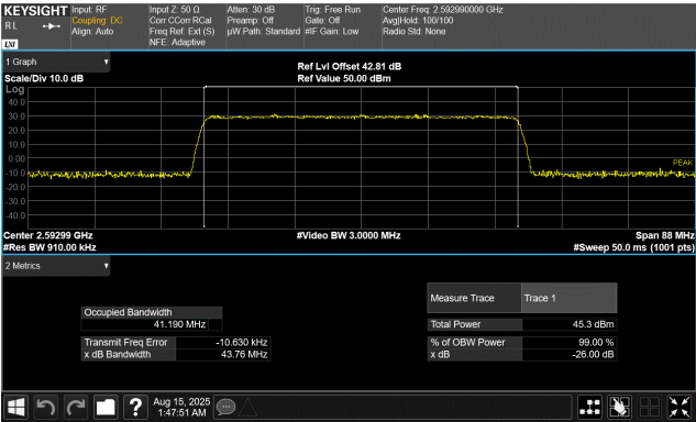
50 MHz Base Channel Bandwidth 44.0 MHz Slim Carrier Bandwidth 256QAM Modulation Middle Channel, 2592.99 MHz
