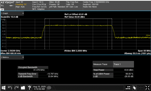
40 MHz Base Channel Bandwidth 34.0 MHz Slim Carrier Bandwidth QPSK Modulation Middle Channel, 2592.99 MHz
