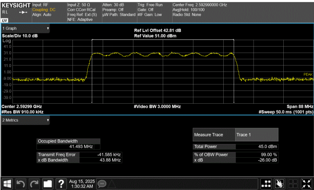
50 MHz Base Channel Bandwidth 44.0 MHz Slim Carrier Bandwidth 16QAM Modulation Middle Channel, 2592.99 MHz
