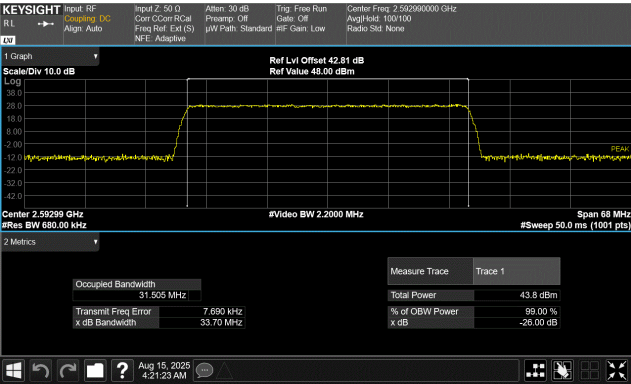
40 MHz Base Channel Bandwidth 34.0 MHz Slim Carrier Bandwidth 64QAM Modulation Middle Channel, 2592.99 MHz
