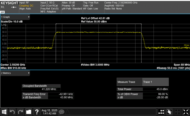
50 MHz Base Channel Bandwidth 44.0 MHz Slim Carrier Bandwidth 64QAM Modulation Middle Channel, 2592.99 MHz
