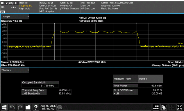
40 MHz Base Channel Bandwidth 34.0 MHz Slim Carrier Bandwidth 16QAM Modulation Middle Channel, 2592.99 MHz
