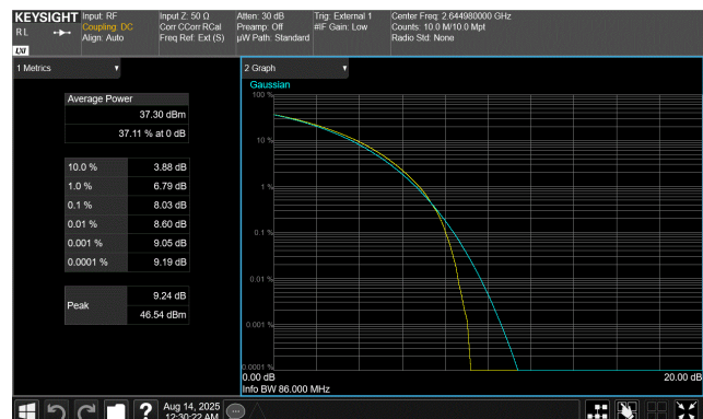
90 MHz Base Channel Bandwidth 86.0 MHz Slim Carrier Bandwidth QPSK Modulation High Channel, 2644.98 MHz
