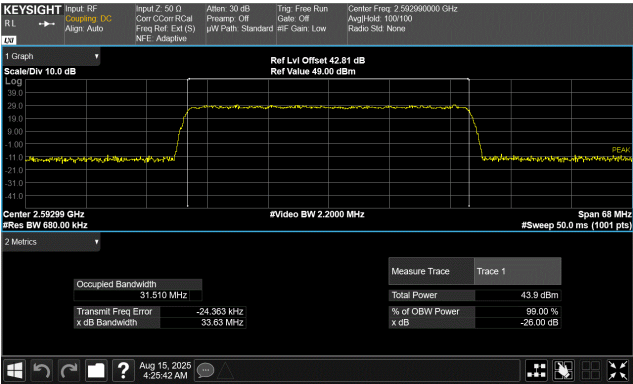
40 MHz Base Channel Bandwidth 34.0 MHz Slim Carrier Bandwidth 256QAM Modulation Middle Channel, 2592.99 MHz
