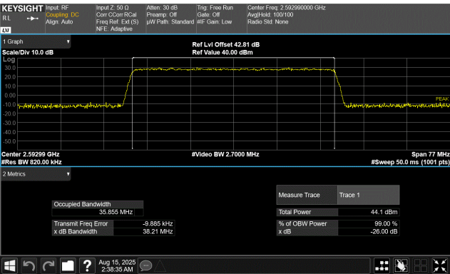
40 MHz Base Channel Bandwidth 38.5 MHz Slim Carrier Bandwidth 64QAM Modulation Middle Channel, 2592.99 MHz
