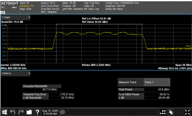
40 MHz Base Channel Bandwidth 33.0 MHz Slim Carrier Bandwidth 16QAM Modulation Middle Channel, 2592.99 MHz
