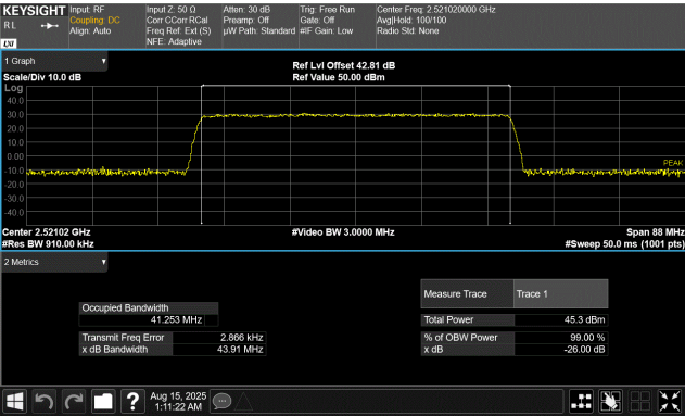
50 MHz Base Channel Bandwidth 44.0 MHz Slim Carrier Bandwidth QPSK Modulation Low Channel, 2521.02 MHz
