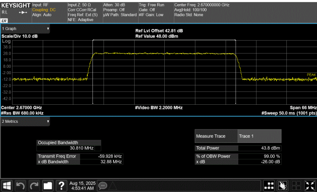
40 MHz Base Channel Bandwidth 33.0 MHz Slim Carrier Bandwidth QPSK Modulation High Channel, 2670.0 MHz
