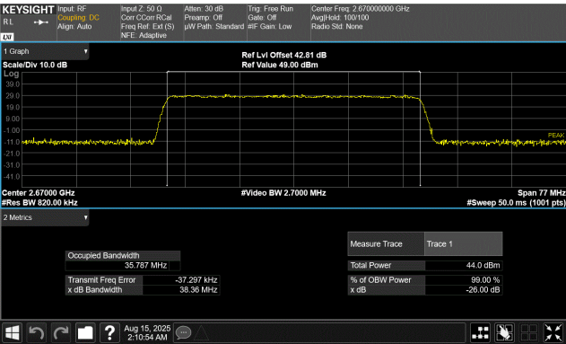
40 MHz Base Channel Bandwidth 38.5 MHz Slim Carrier Bandwidth QPSK Modulation High Channel, 2670.0 MHz
