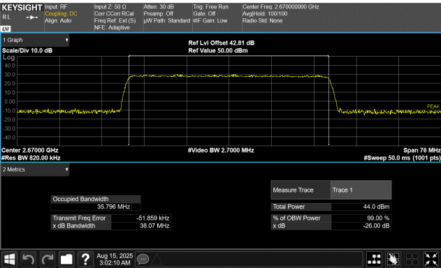
40 MHz Base Channel Bandwidth 38.0 MHz Slim Carrier Bandwidth QPSK Modulation High Channel, 2670.0 MHz
