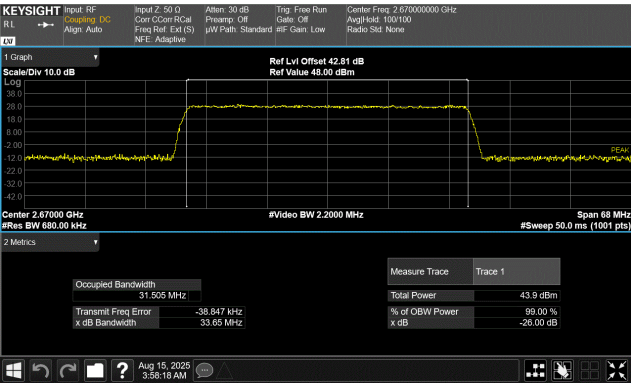
40 MHz Base Channel Bandwidth 34.0 MHz Slim Carrier Bandwidth QPSK Modulation High Channel, 2670.0 MHz
