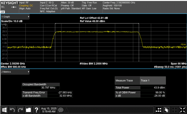
40 MHz Base Channel Bandwidth 33.0 MHz Slim Carrier Bandwidth 256QAM Modulation Middle Channel, 2592.99 MHz
