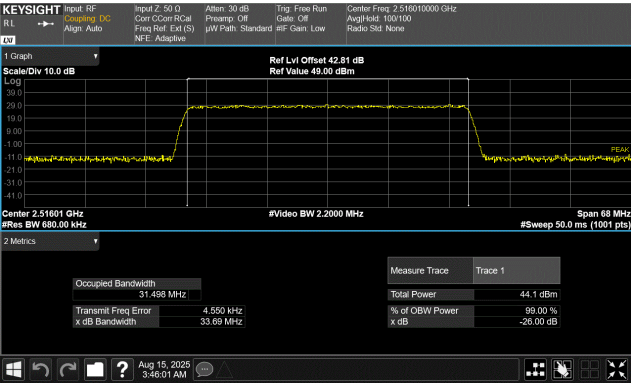
40 MHz Base Channel Bandwidth 34.0 MHz Slim Carrier Bandwidth QPSK Modulation Low Channel, 2516.01 MHz
