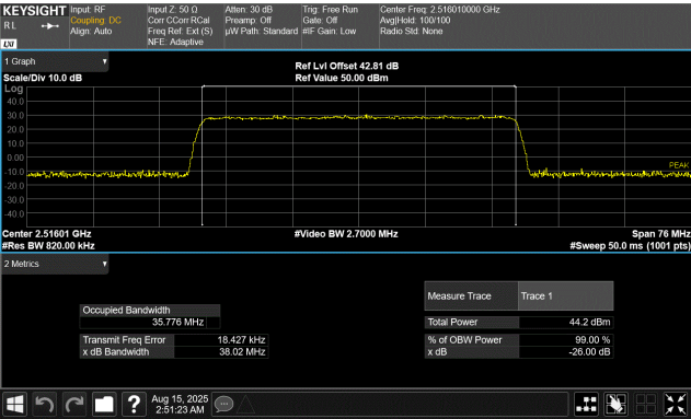
40 MHz Base Channel Bandwidth 38.0 MHz Slim Carrier Bandwidth QPSK Modulation Low Channel, 2516.01 MHz
