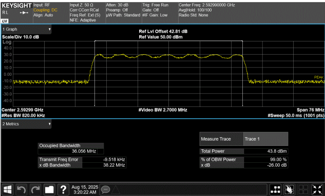
40 MHz Base Channel Bandwidth 38.0 MHz Slim Carrier Bandwidth 16QAM Modulation Middle Channel, 2592.99 MHz
