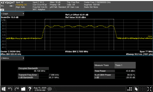
40 MHz Base Channel Bandwidth 38.5 MHz Slim Carrier Bandwidth 16QAM Modulation Middle Channel, 2592.99 MHz
