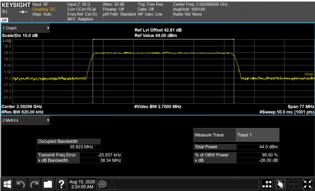
40 MHz Base Channel Bandwidth 38.5 MHz Slim Carrier Bandwidth QPSK Modulation Middle Channel, 2592.99 MHz
