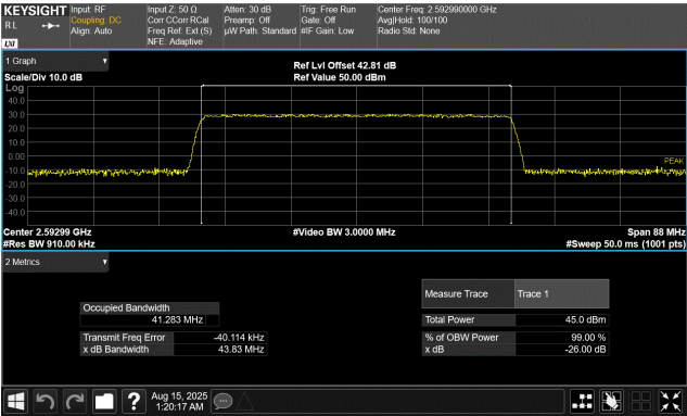
50 MHz Base Channel Bandwidth 44.0 MHz Slim Carrier Bandwidth QPSK Modulation Middle Channel, 2592.99 MHz
