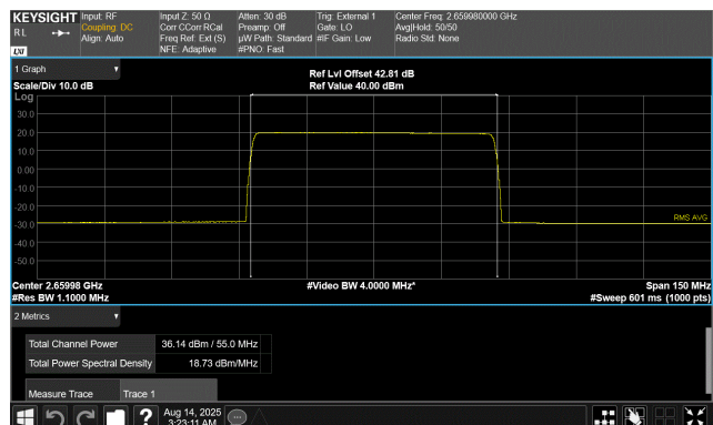
60 MHz Base Channel Bandwidth 55.0 MHz Slim Carrier Bandwidth QPSK Modulation High Channel, 2659.98 MHz
