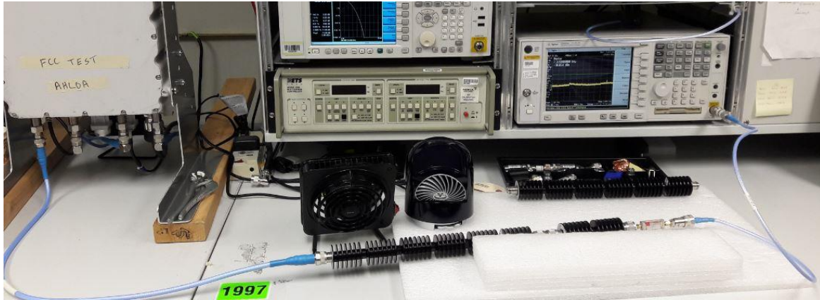
Photograph of 1.1GHz to 8GHz Test Setup
